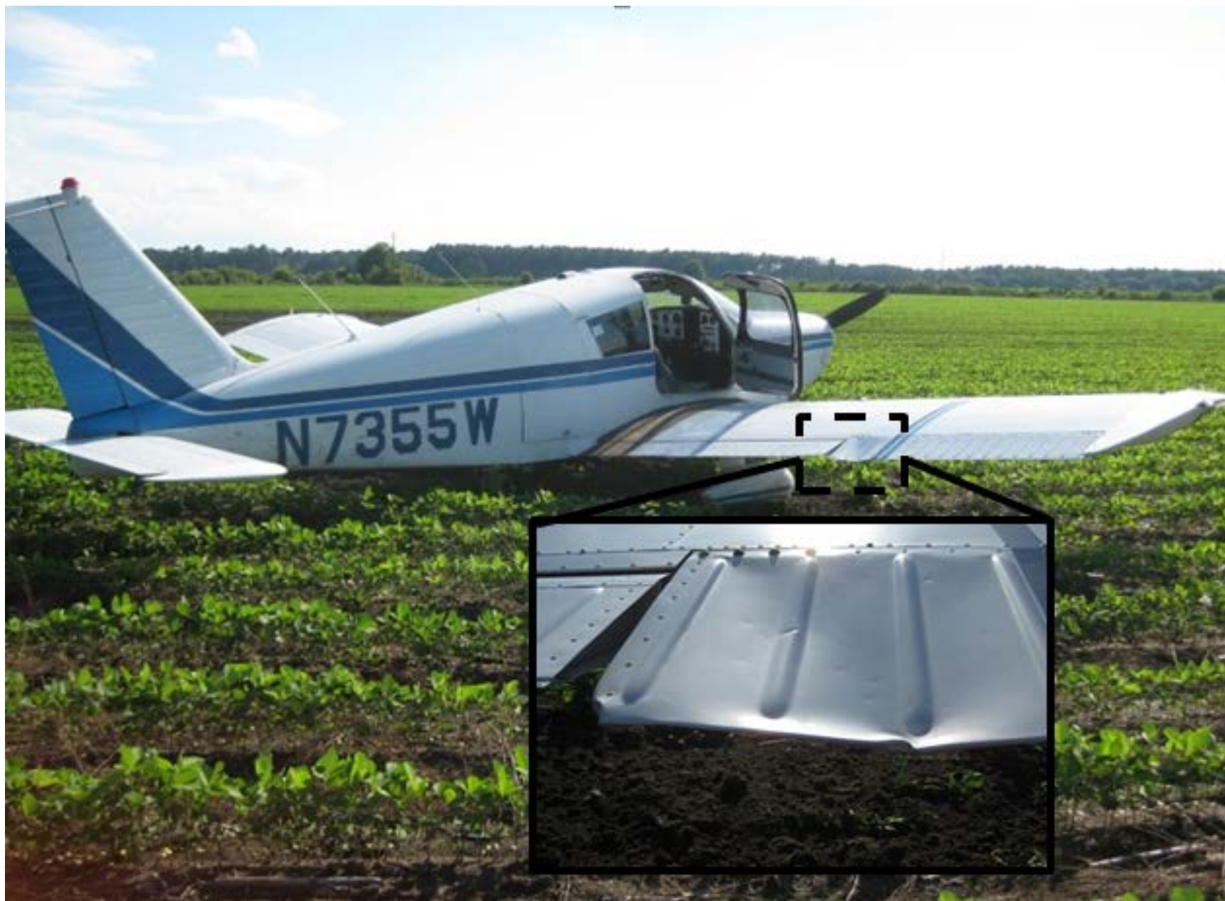
Photo 1 – View of damaged right aileron (photo courtesy of the FAA)
