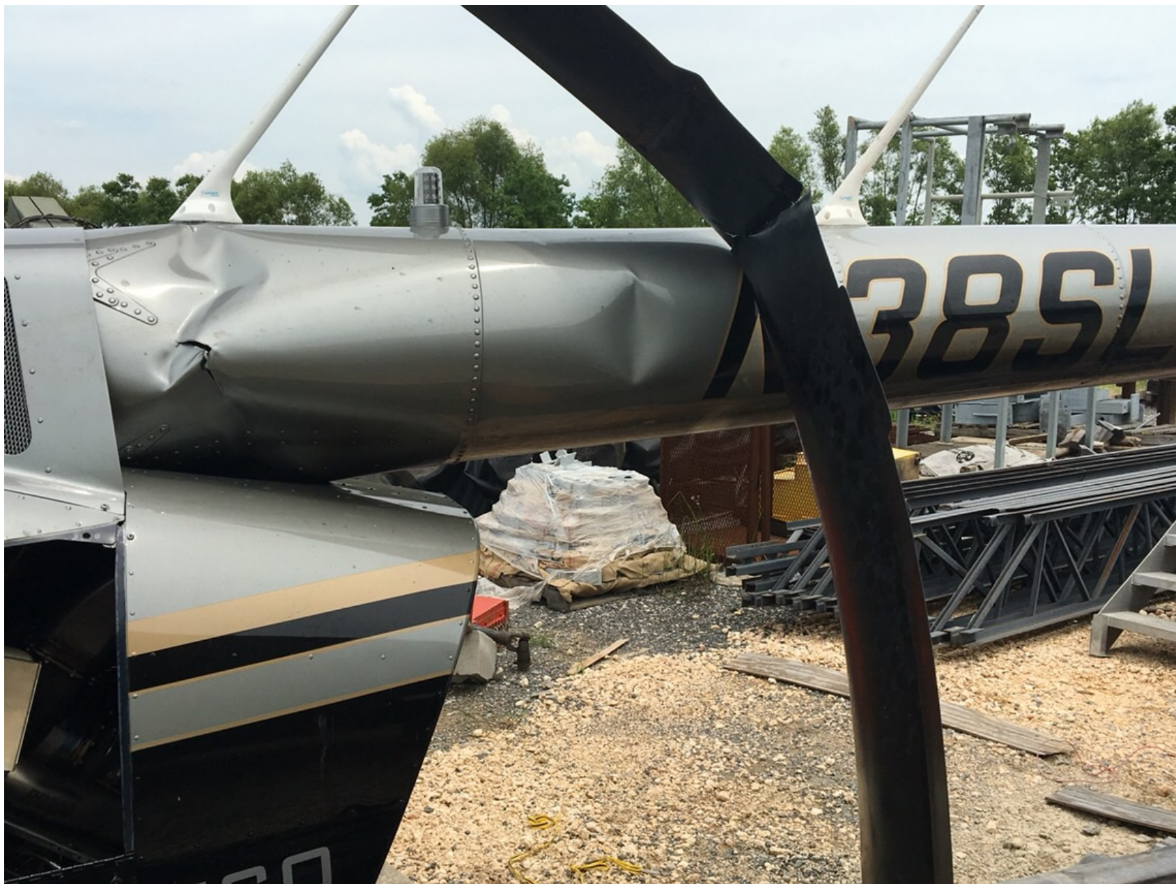
Photo 2 – Substantially Damaged Tail Boom (Photo Courtesy of FAA)
