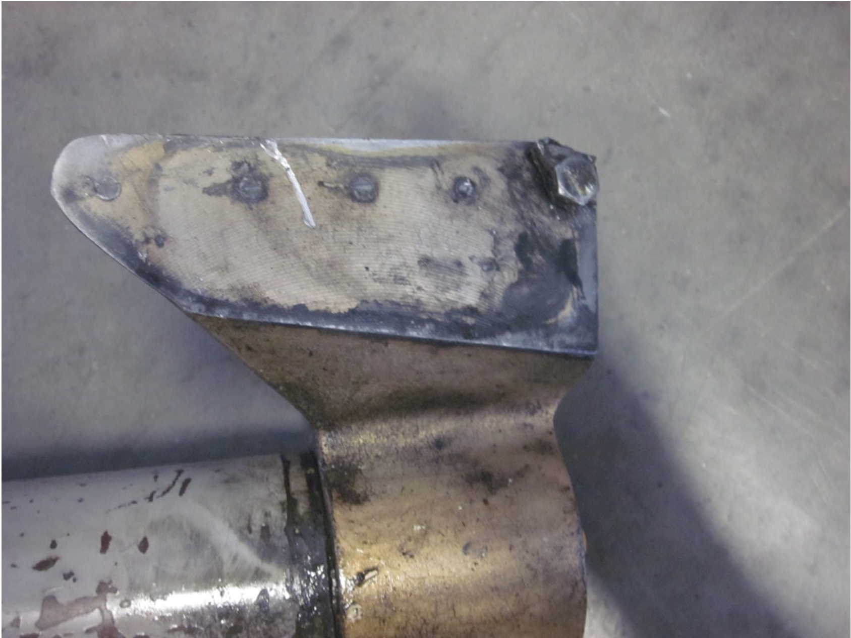
Photo 5 – Failed upper forging (Courtesy of FAA)
