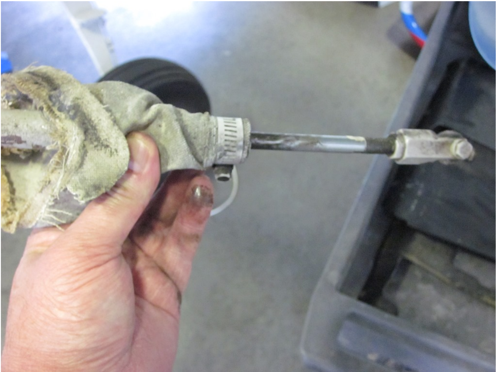
Photo 10 – Failed steering bungee (Courtesy of FAA)
