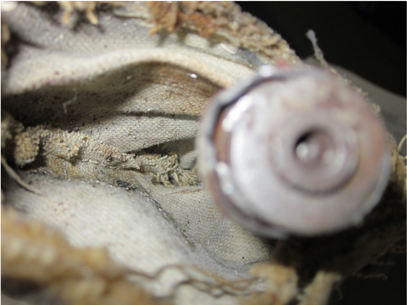
Photo 12 – Aft end of steering bungee fracture surface (Courtesy of FAA)
