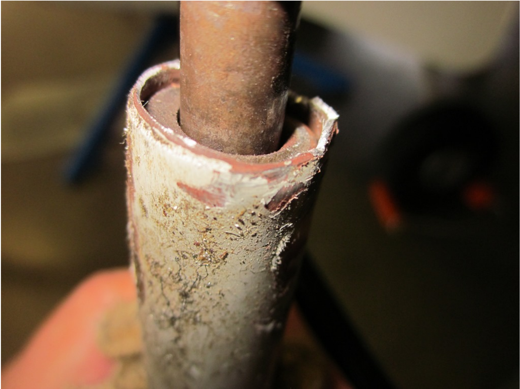
Photo 11 – Steering bungee tube fracture surface (Courtesy of FAA)
