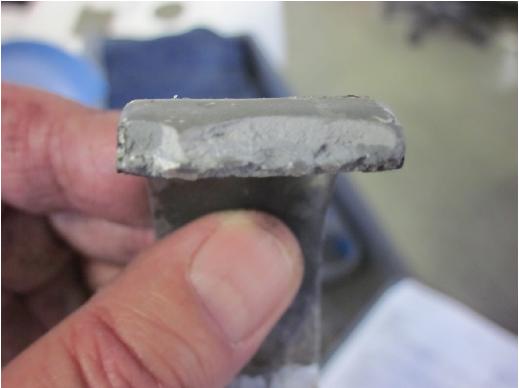
Photo 7 – Failed lower forging clamp (Courtesy of FAA)
