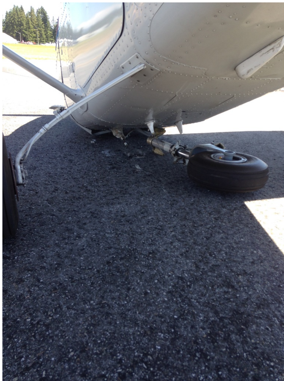
Photo 3 – Collapsed nose gear strut assembly (Courtesy of FAA)
