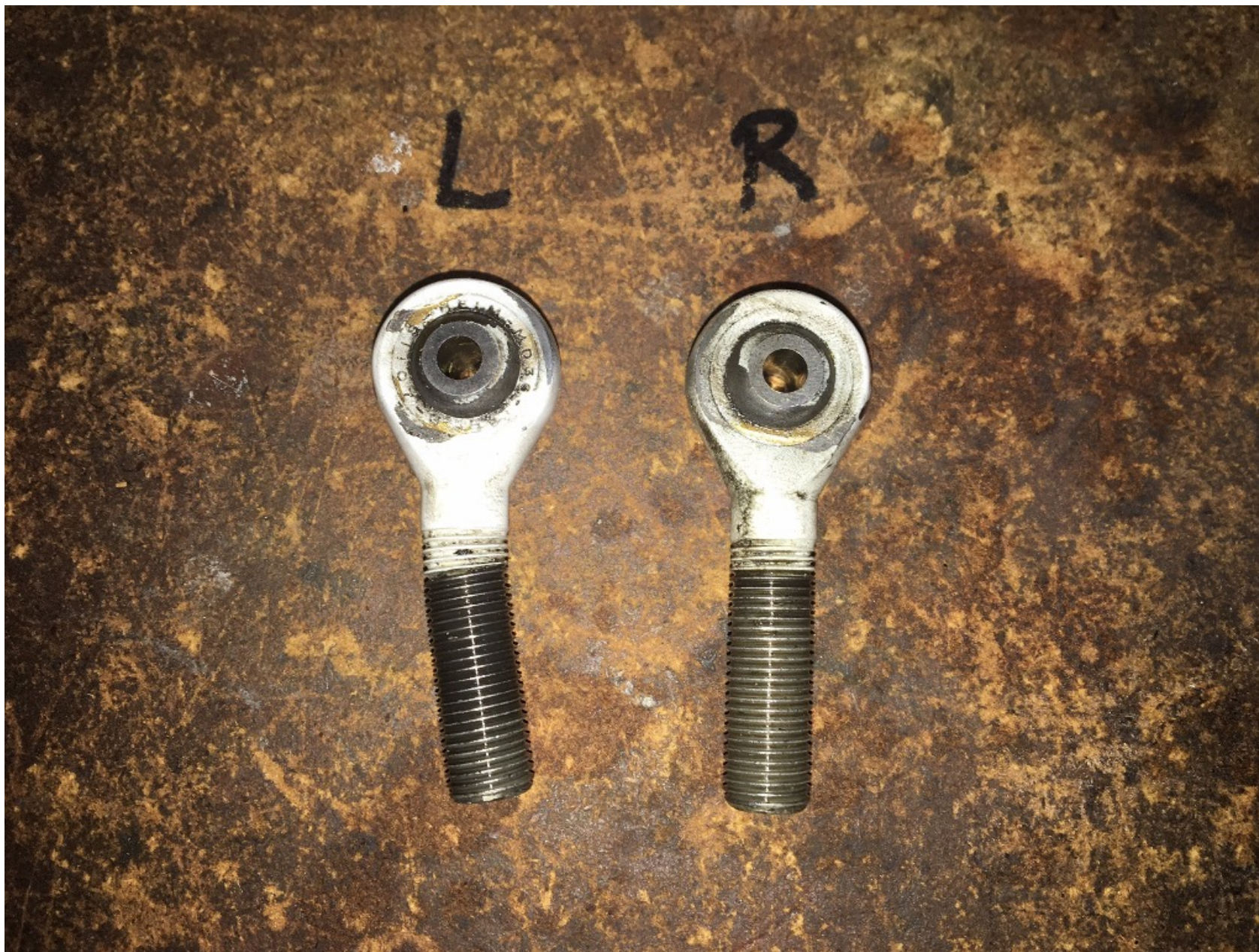
Photo 14 – Steering rod ends from second non-accident C-172 with visible bending of left rod end (Courtesy of operator)
