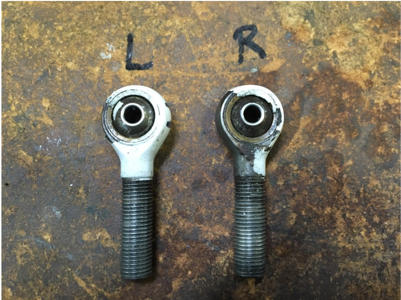
Photo 13 -Steering rod ends from first non-accident C-172 with visible bending of right rod end (Courtesy of operator) □
