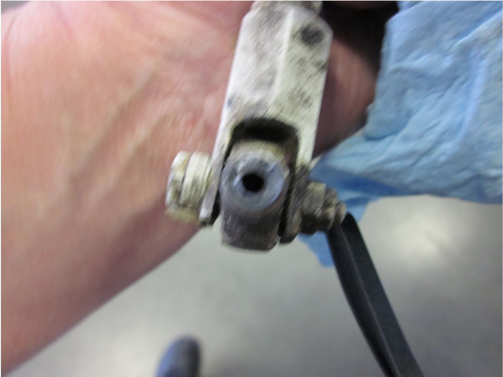
Photo 9 – Failed steering rod end attached steering tube clevis (Courtesy of FAA)
