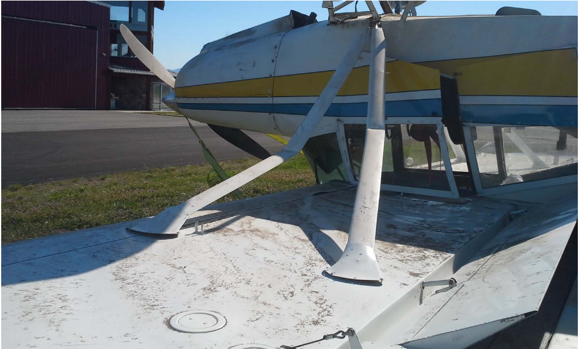
Photo 1 – View of right lift strut damage (Photo Courtesy of FAA)
