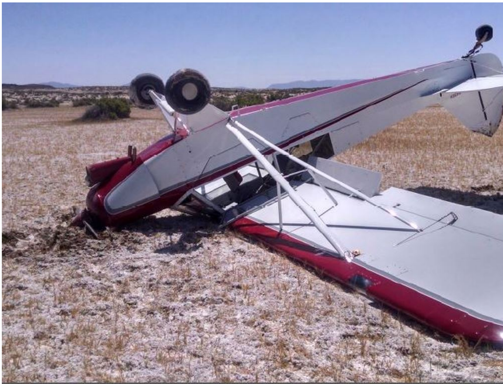
Photo 1 – View of substantial damage to rudder (Courtesy of Pilot)
