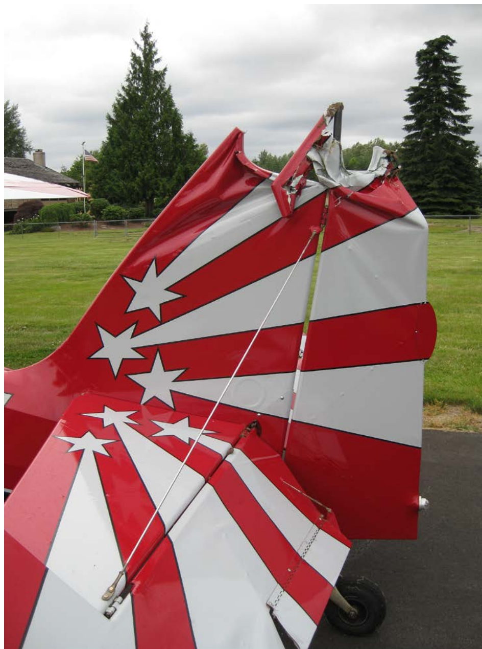
Photo 1 – View of damaged empennage (photo courtesy of the FAA)
