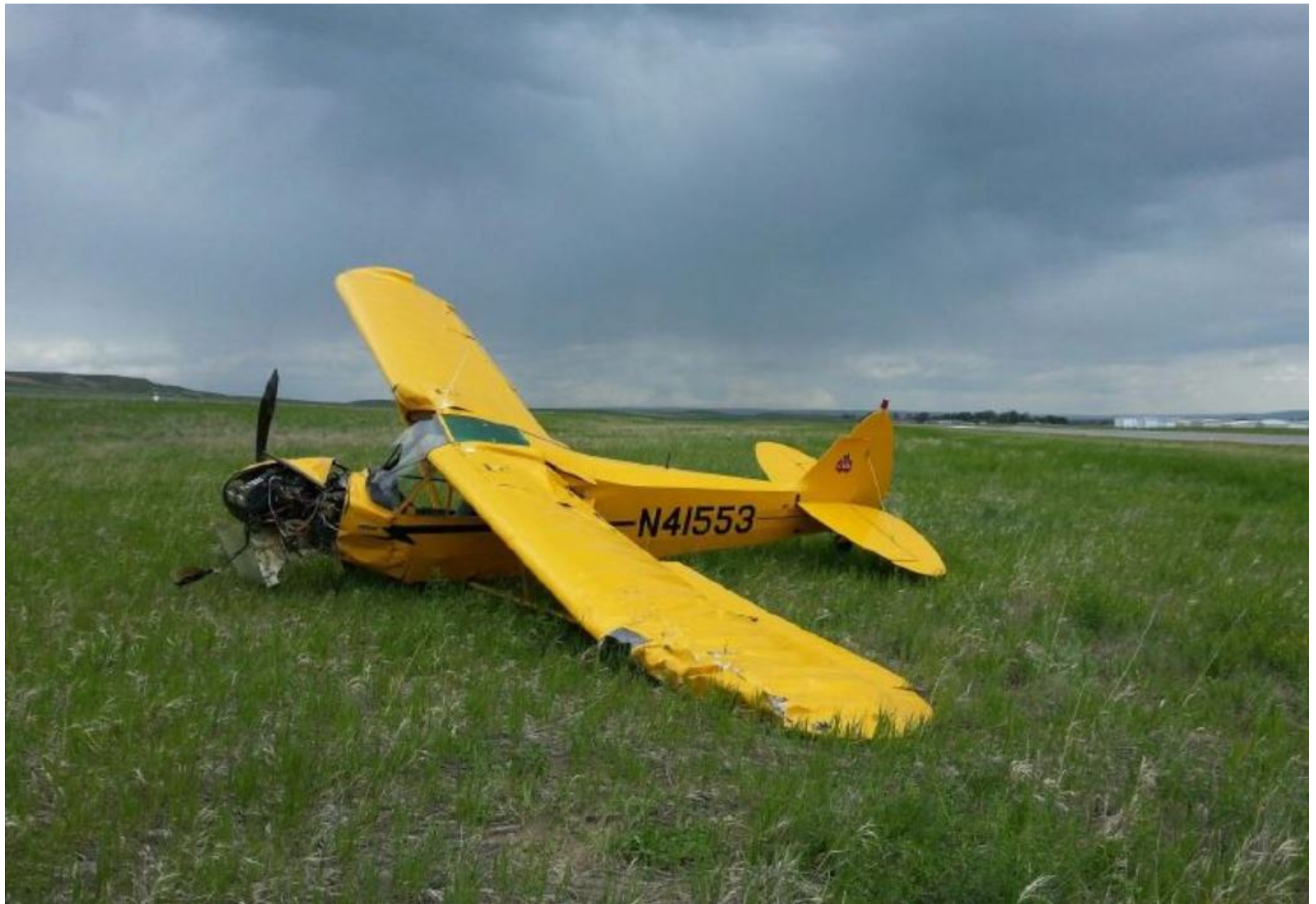
Photo 1 – View of damage to both wings (Courtesy of FAA)
