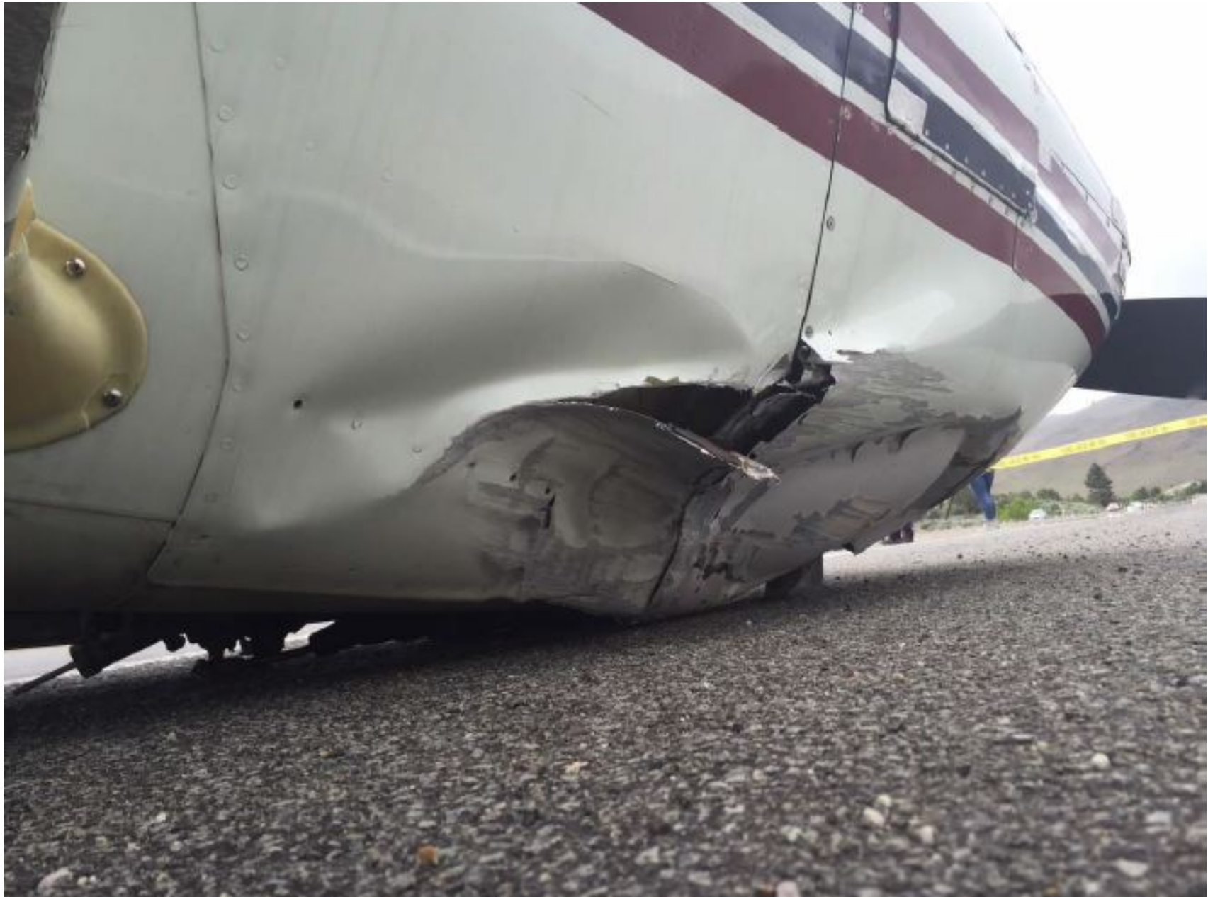
Photo 1 – View of substantial damage to firewall (Courtesy of FAA)
