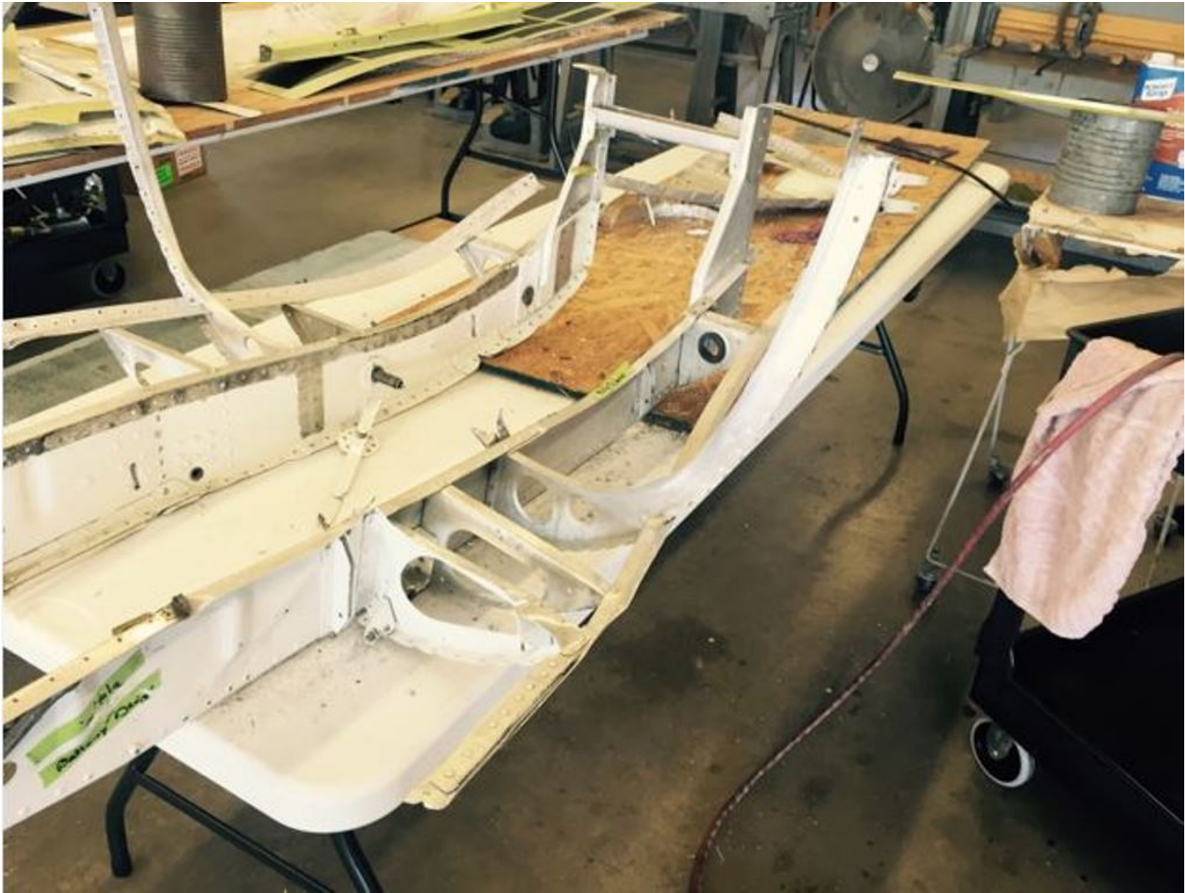
Photo 1 – View of substantial damage to keel beams (Courtesy of Repair Facility)
