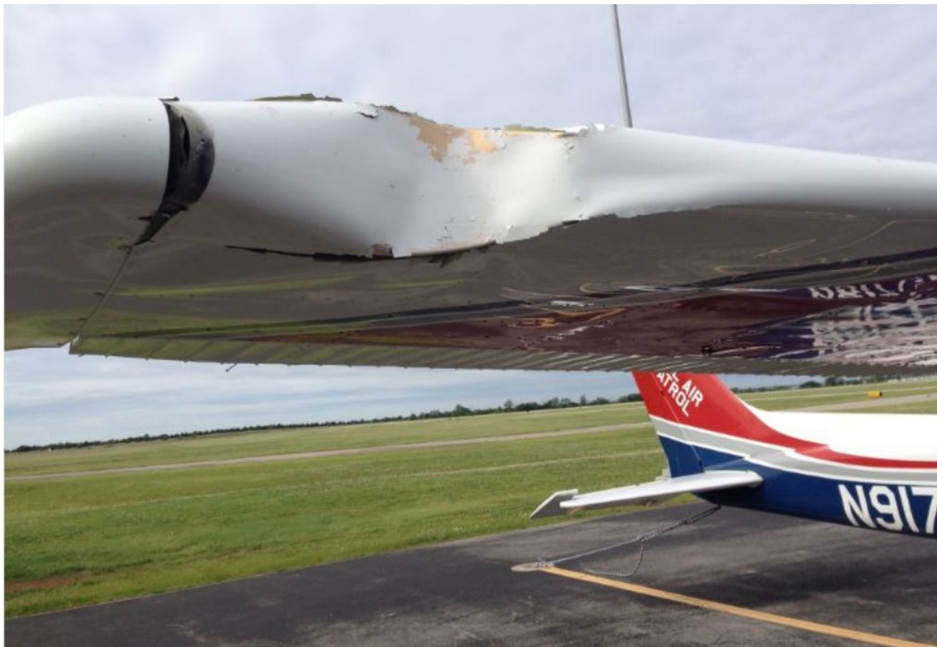
Photo 1 – View of damage to right wing rib and spar (Courtesy of FAA)
