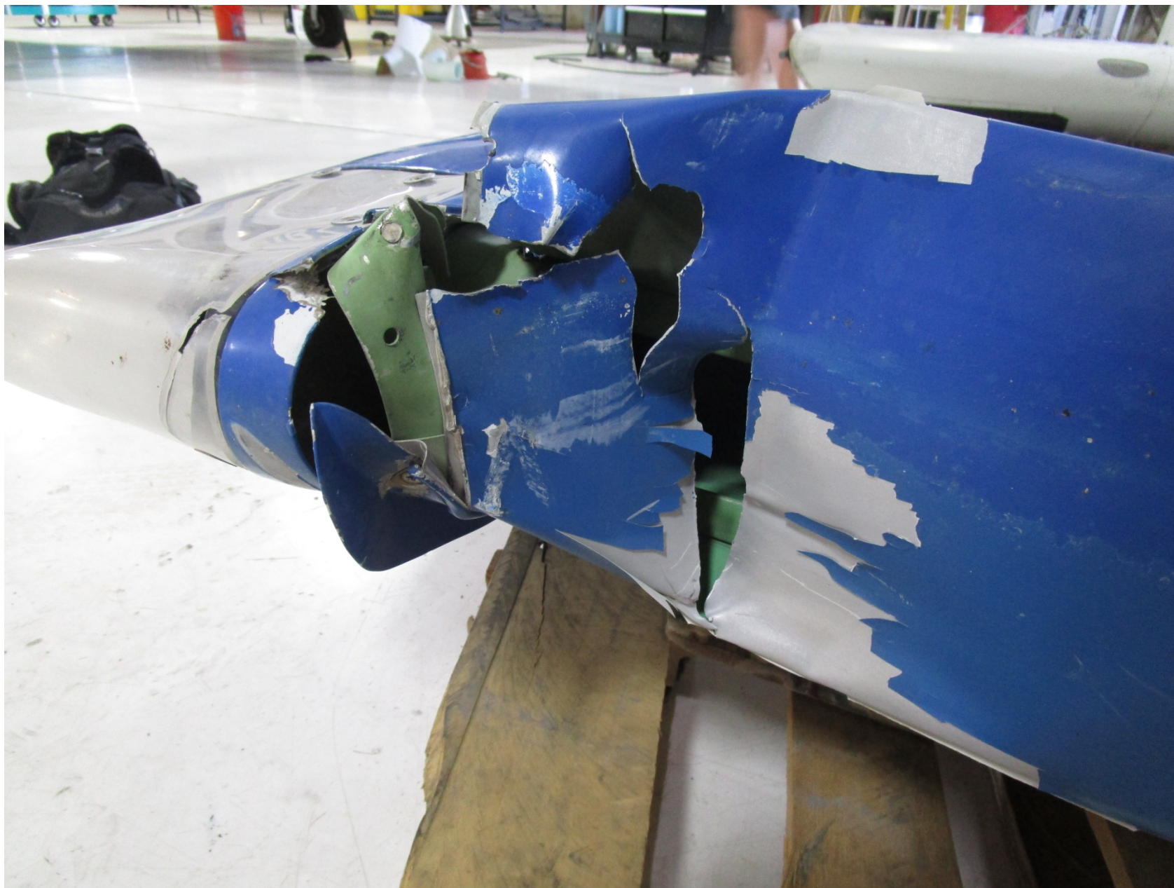
Photo 2 – Left Wing Spar Damage (Photo Courtesy of FAA)
