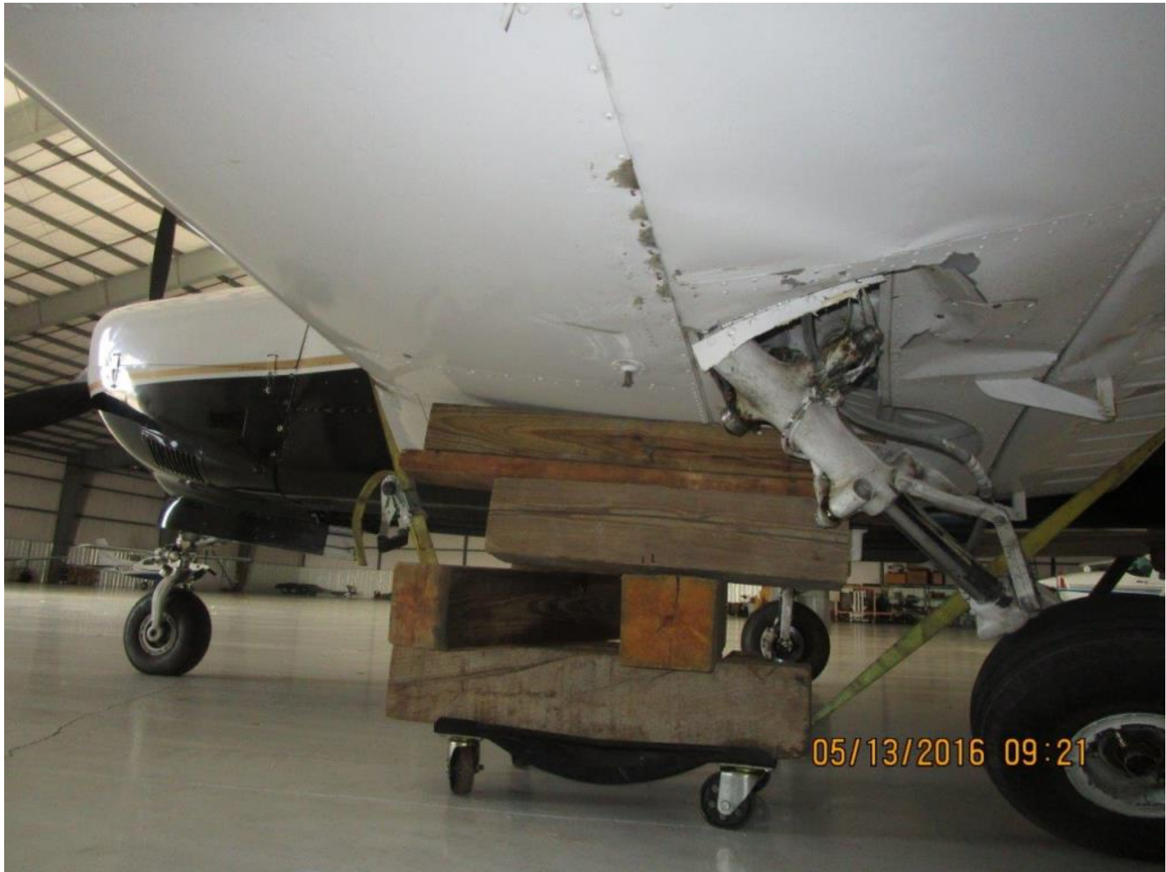
Photo 1 – View of substantial damage to left flap and landing gear attachment fitting (Courtesy of FAA)
