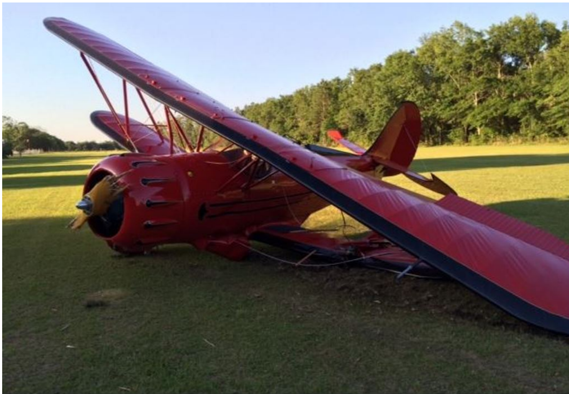
Photo 1 – View of substantial damage to left wings and fuselage (Courtesy of Pilot)
