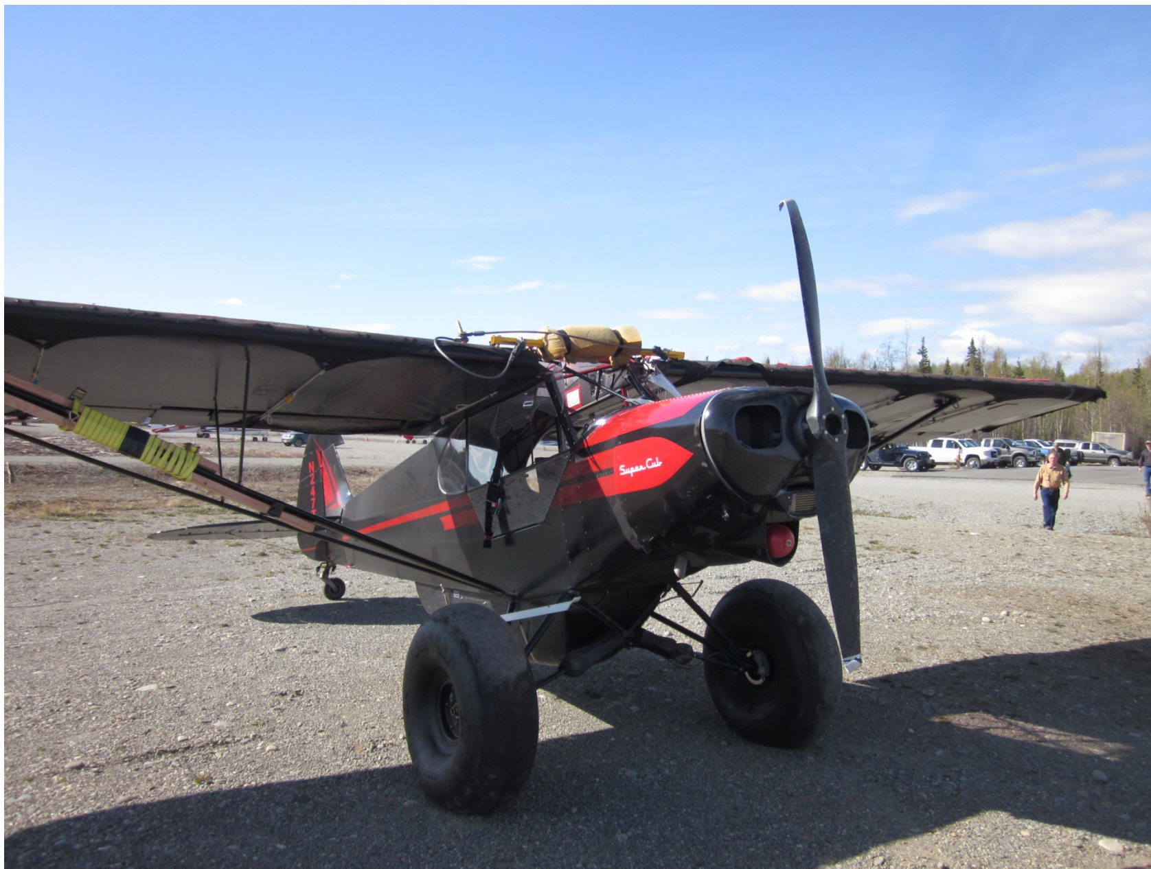
Photo 1 – View of substantially damaged windscreen and right wing lift strut (photo courtesy of FAA)
