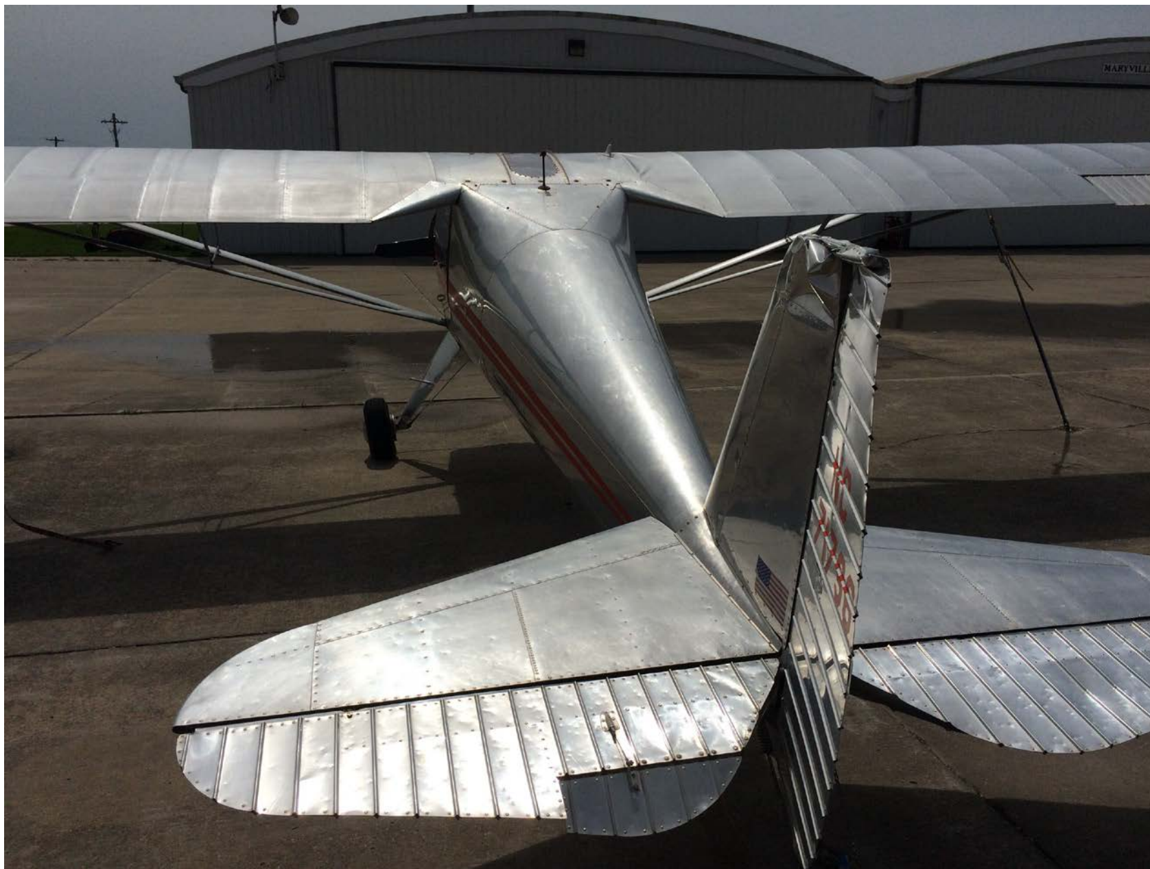
Photo 1 – Substantially Damaged Vertical Stabilizer and Rudder (Photo courtesy of FAA)
