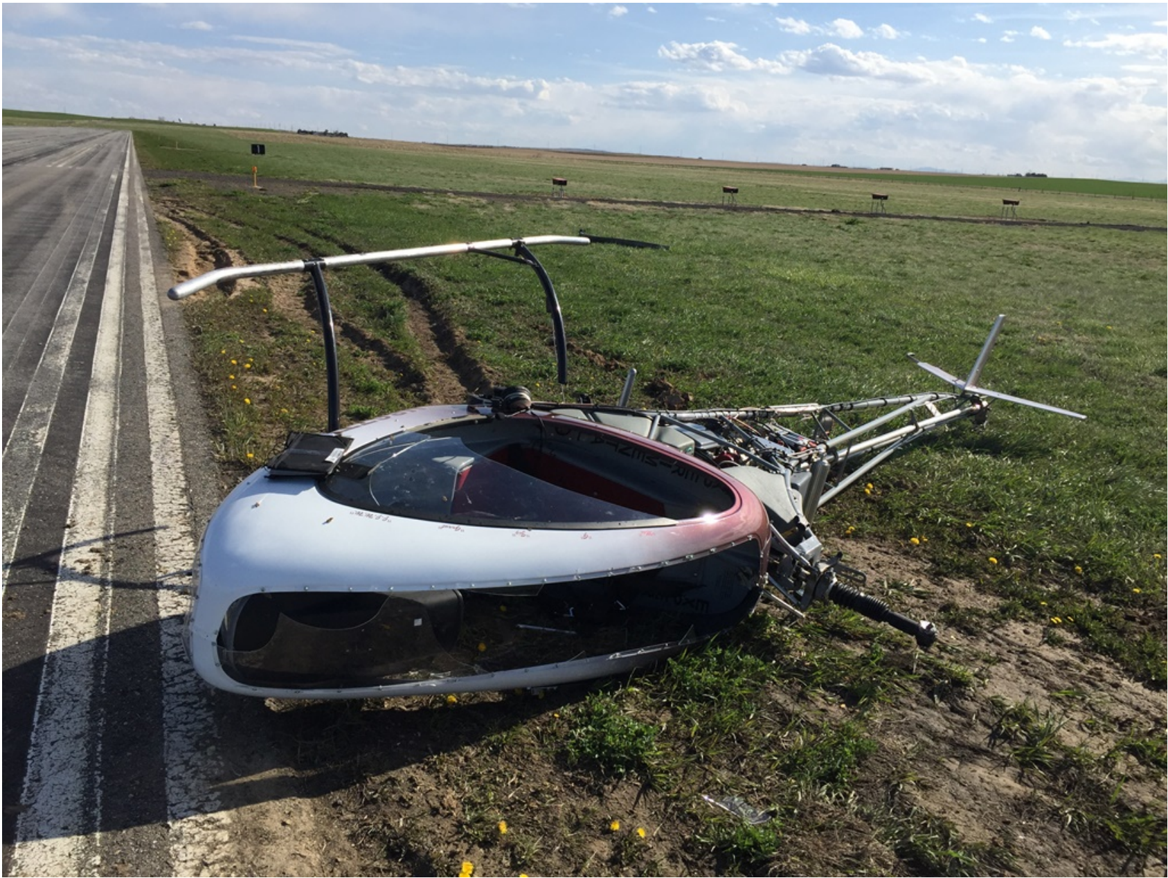
Photo 1 – View of damage to wind screen and rotor systems (Courtesy of FAA)
