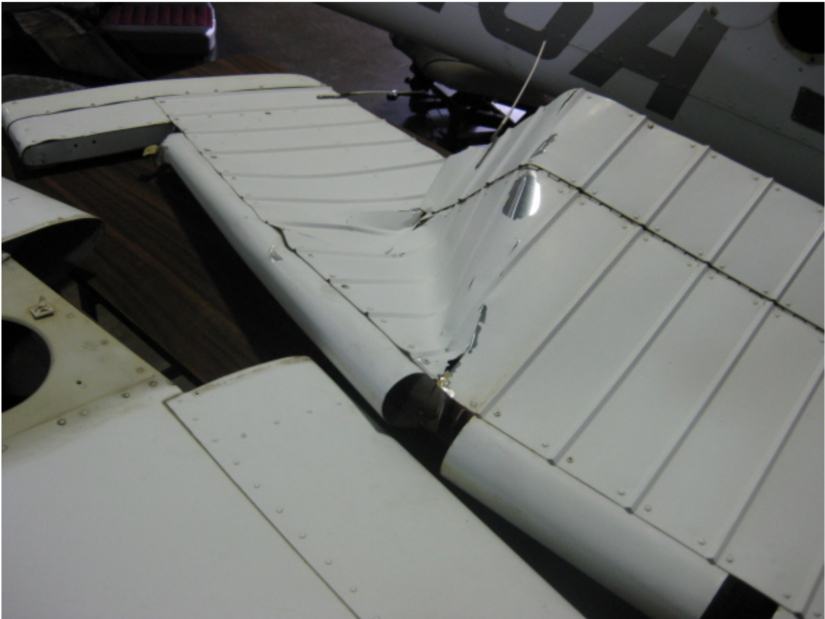
Photo 1 – View of the substantially damaged elevator (Photo courtesy of FAA)
