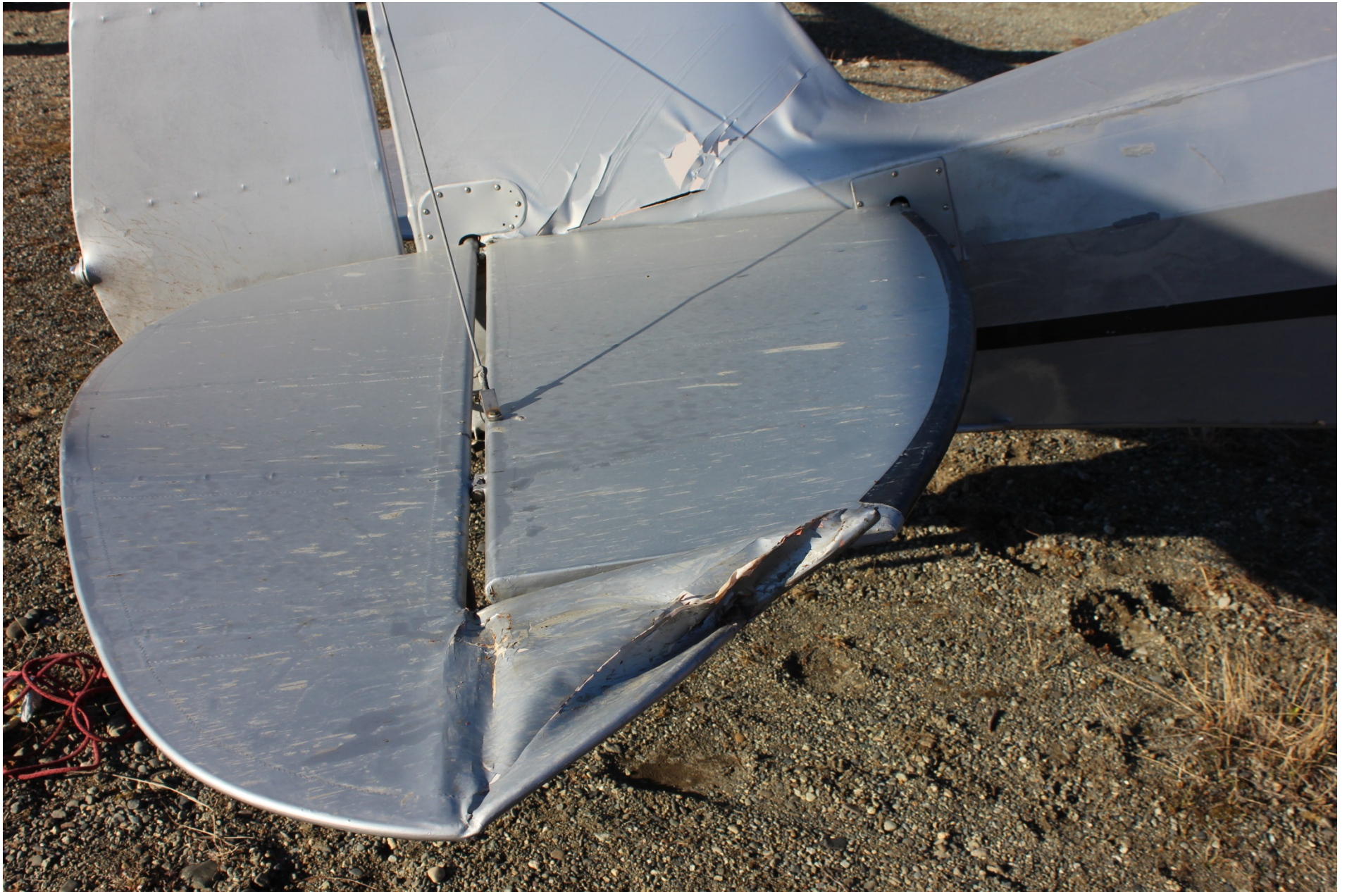
Photo 1 – View of damaged empennage (photo courtesy of the FAA)
