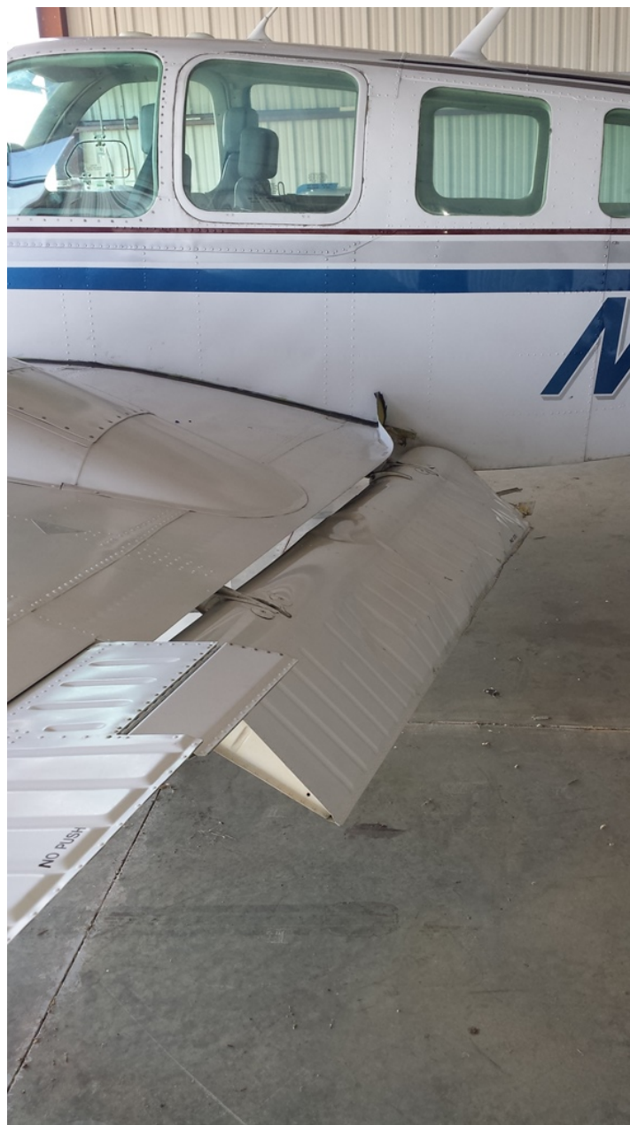
Photo 3 – View of damage to the inboard left wing and left aileron (Courtesy of FAA)
