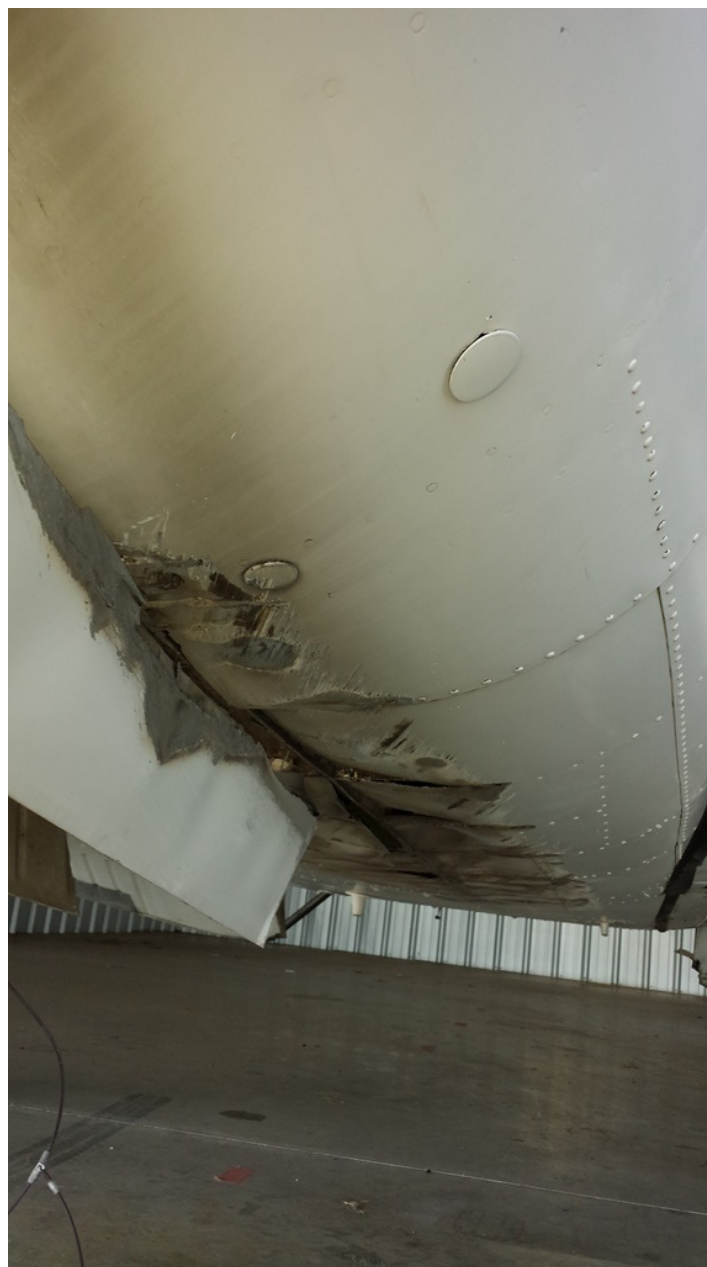
Photo 2 – View of damage to the bottom of the fuselage (Courtesy of FAA)
