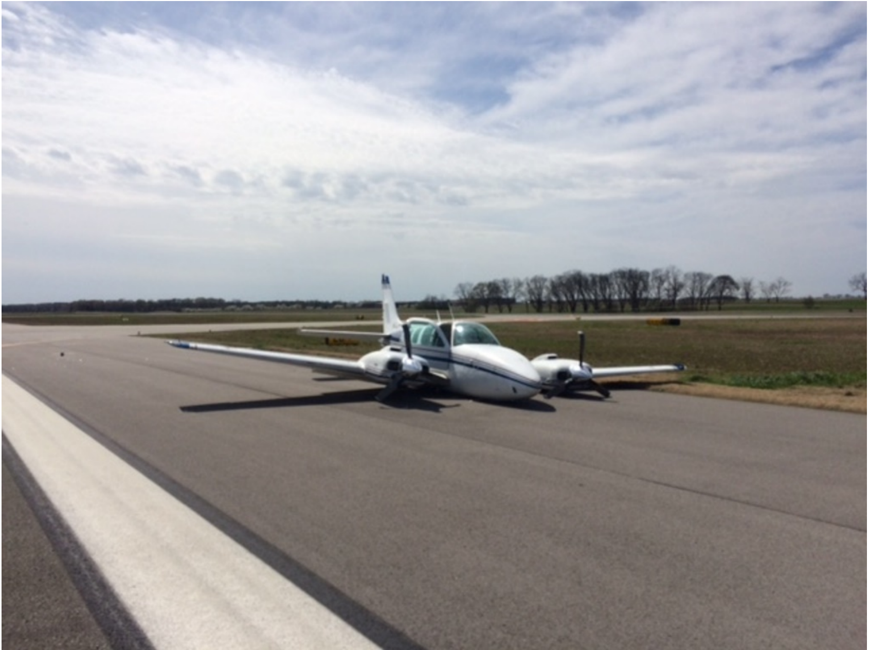
Photo 1 – View of the airplane on the runway with retracted landing gear (Courtesy of FAA)
