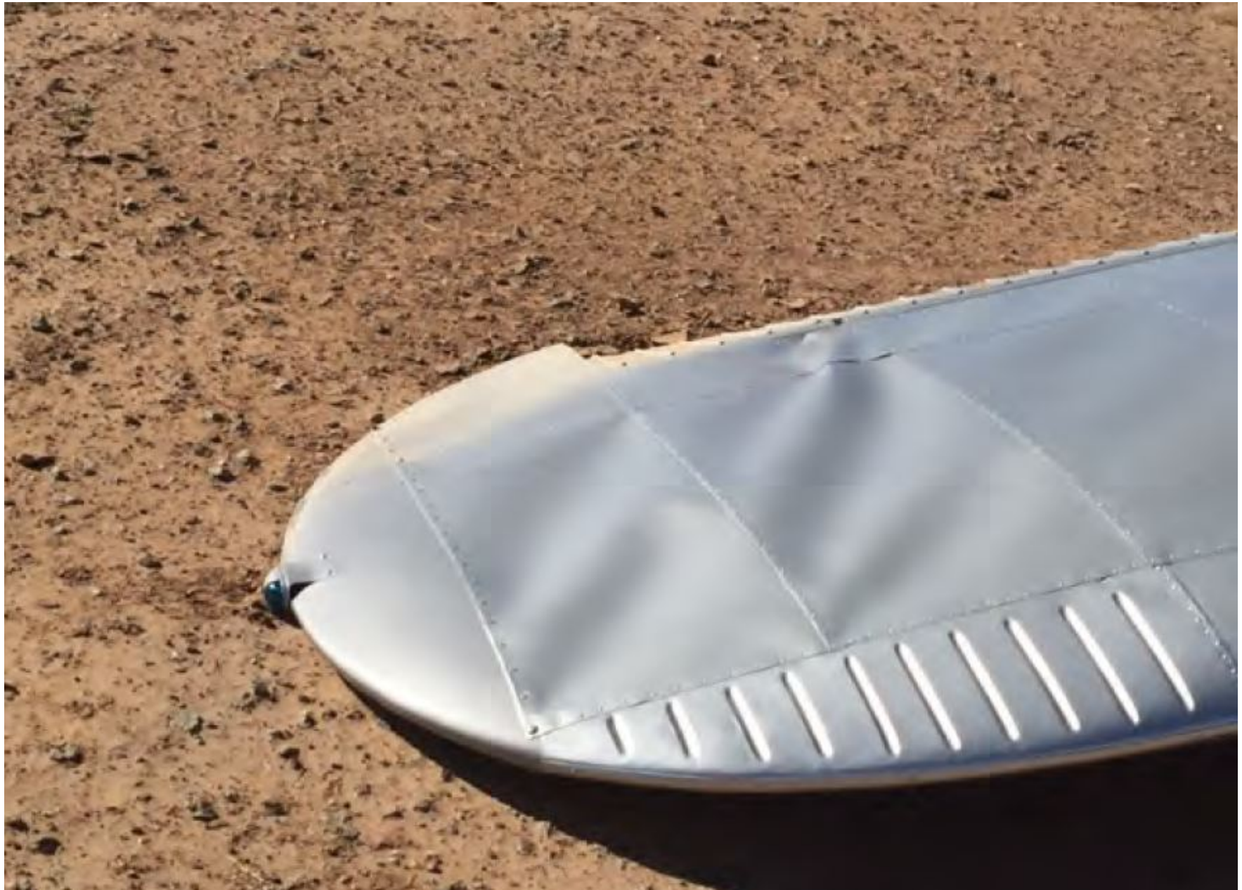
Photo 2 – Substantial Damage to Right Wing (Courtesy of FAA)
