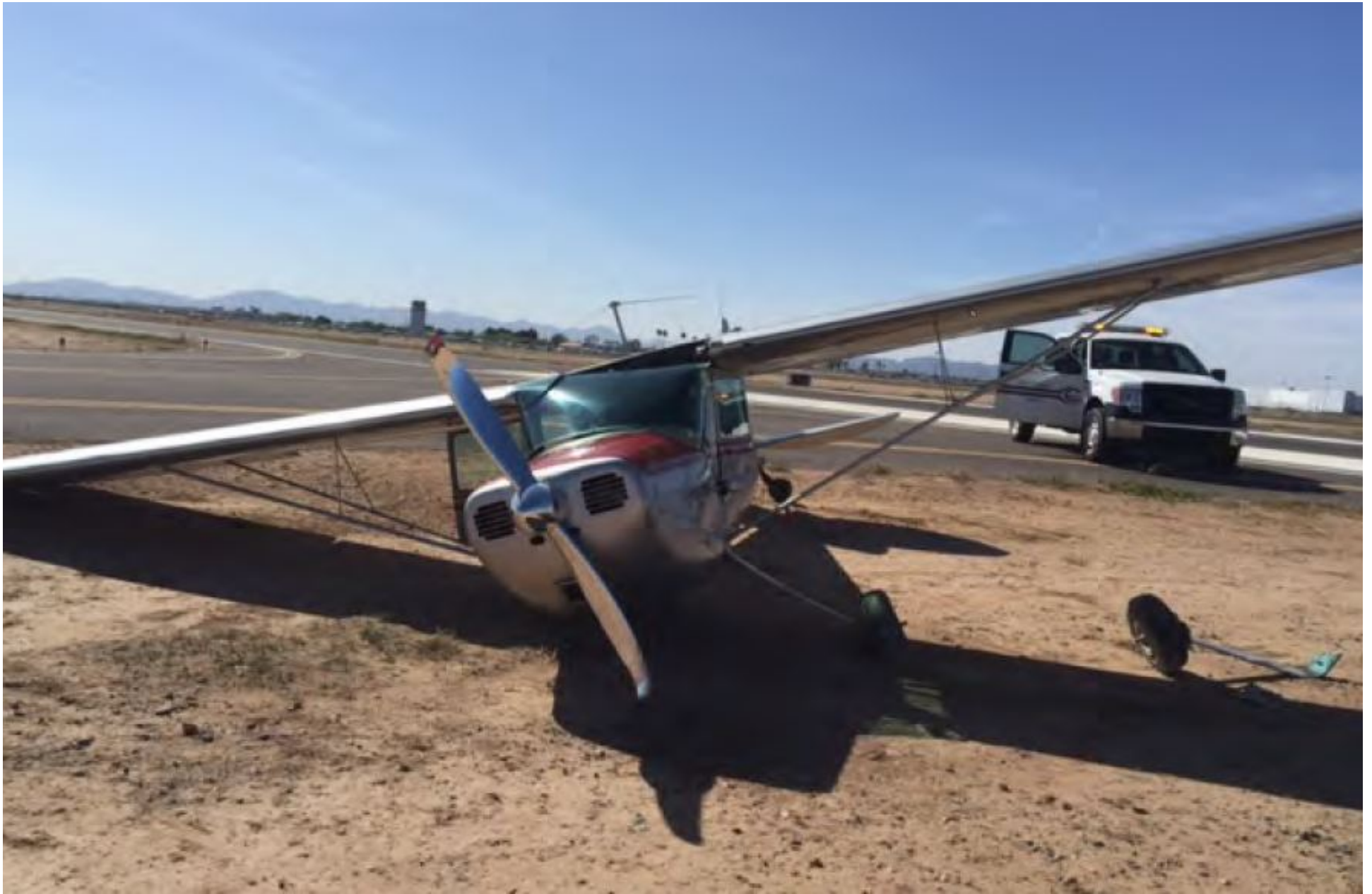
Photo 1 – Airplane with Collapsed Right Main Landing Gear (Courtesy of FAA)
