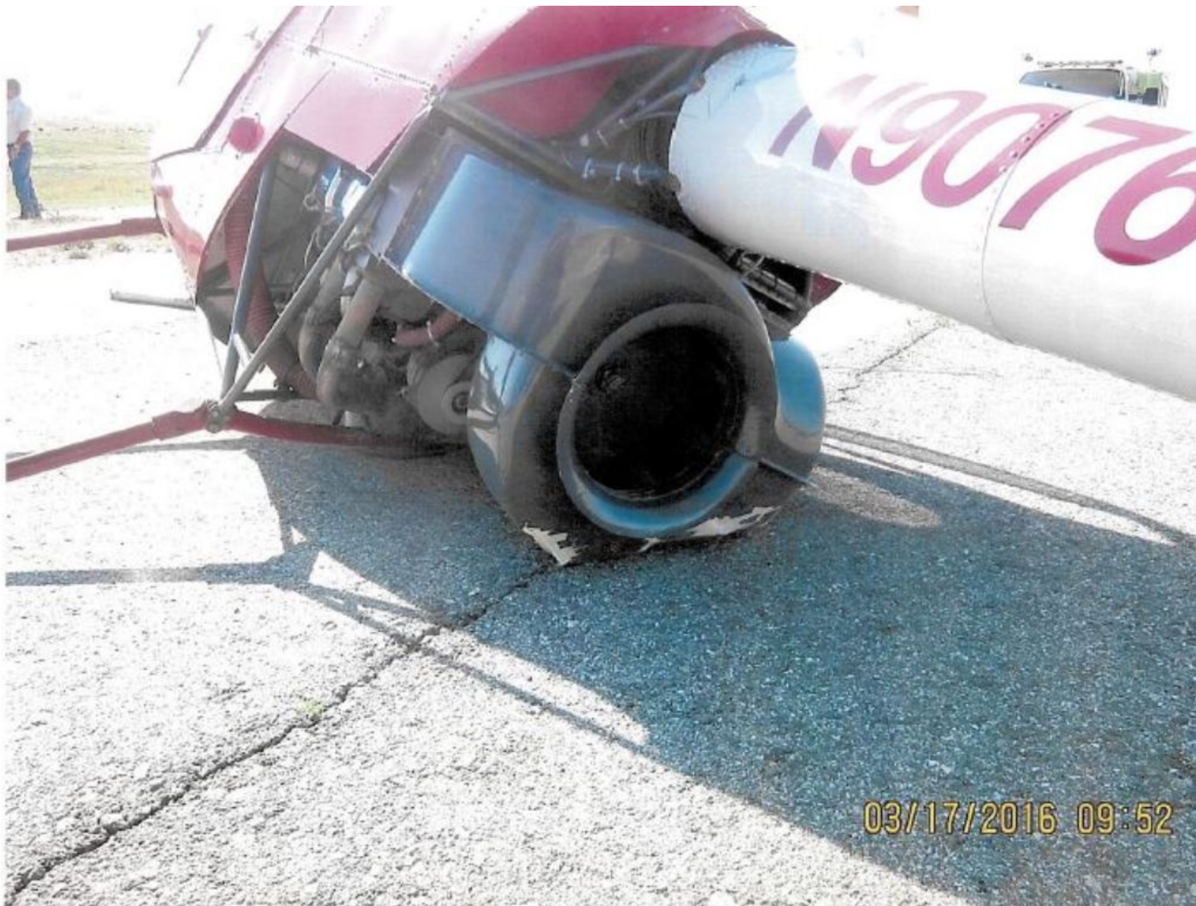
Photo 1 – View of damage to the helicopter frame (Courtesy of FAA)
