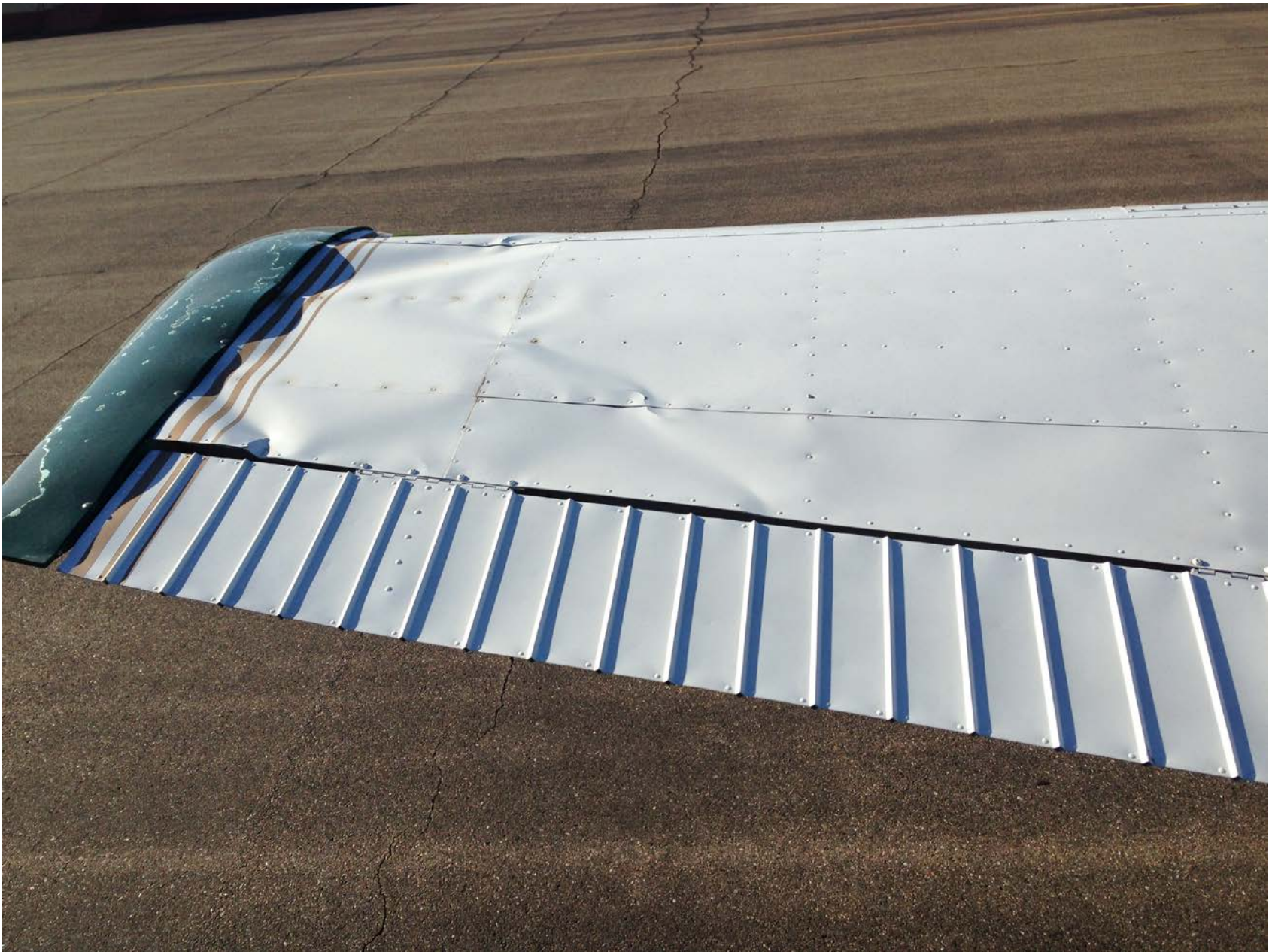
Photo 2 - View of left wing damage from rear (report courtesy of the FAA)
