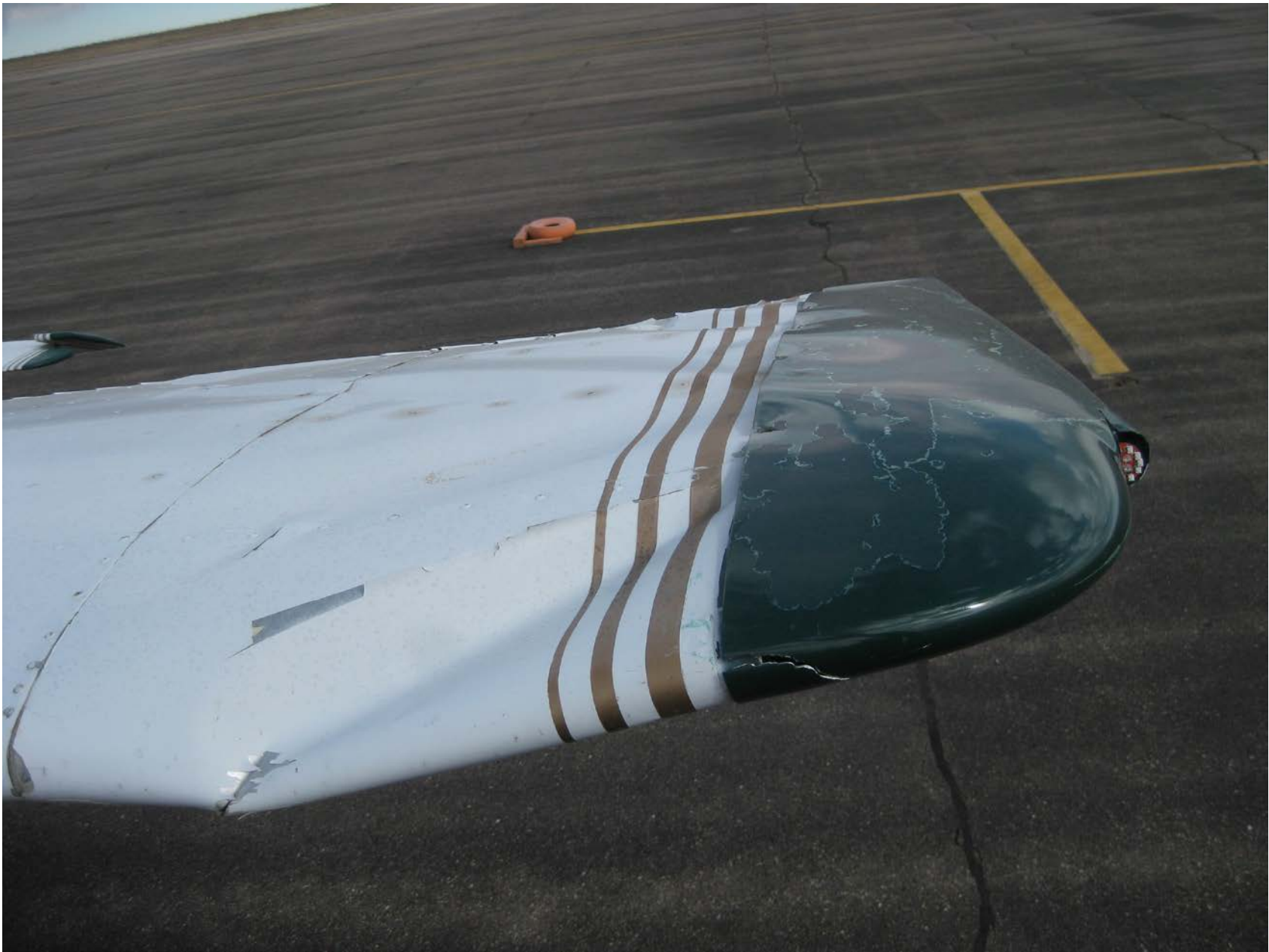
Photo 1 – View of left wing damage from front (report courtesy of the FAA)
