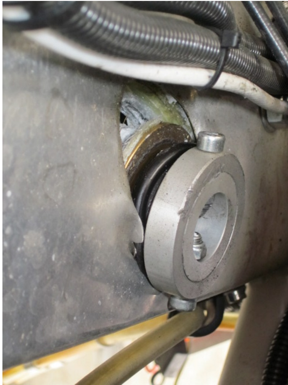
Photo 2 – View of substantial damage to firewall (Courtesy of FAA)
