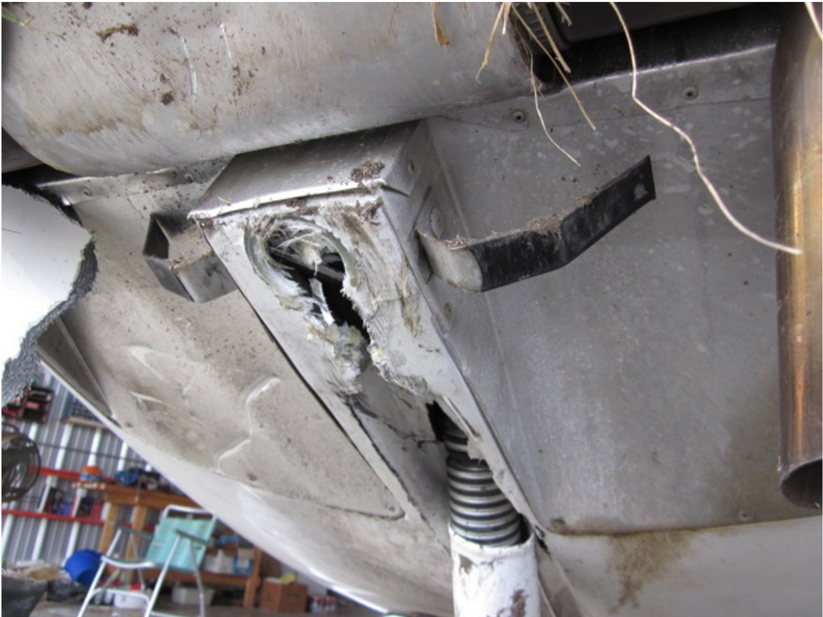
Photo 1 – View of damage to composite fuselage (Courtesy of FAA)
