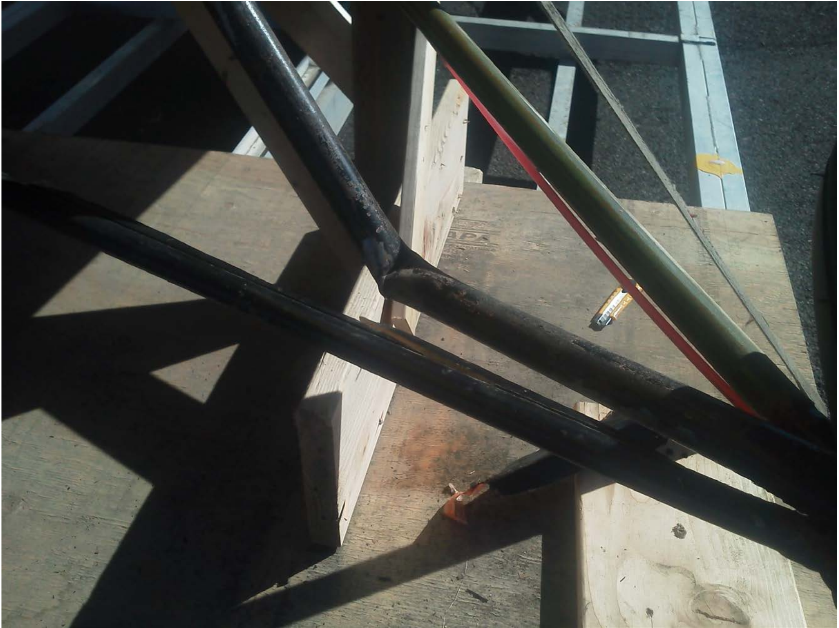
Photo 2 -View of left main landing forward gear tube (photo courtesy of the Pilot)
