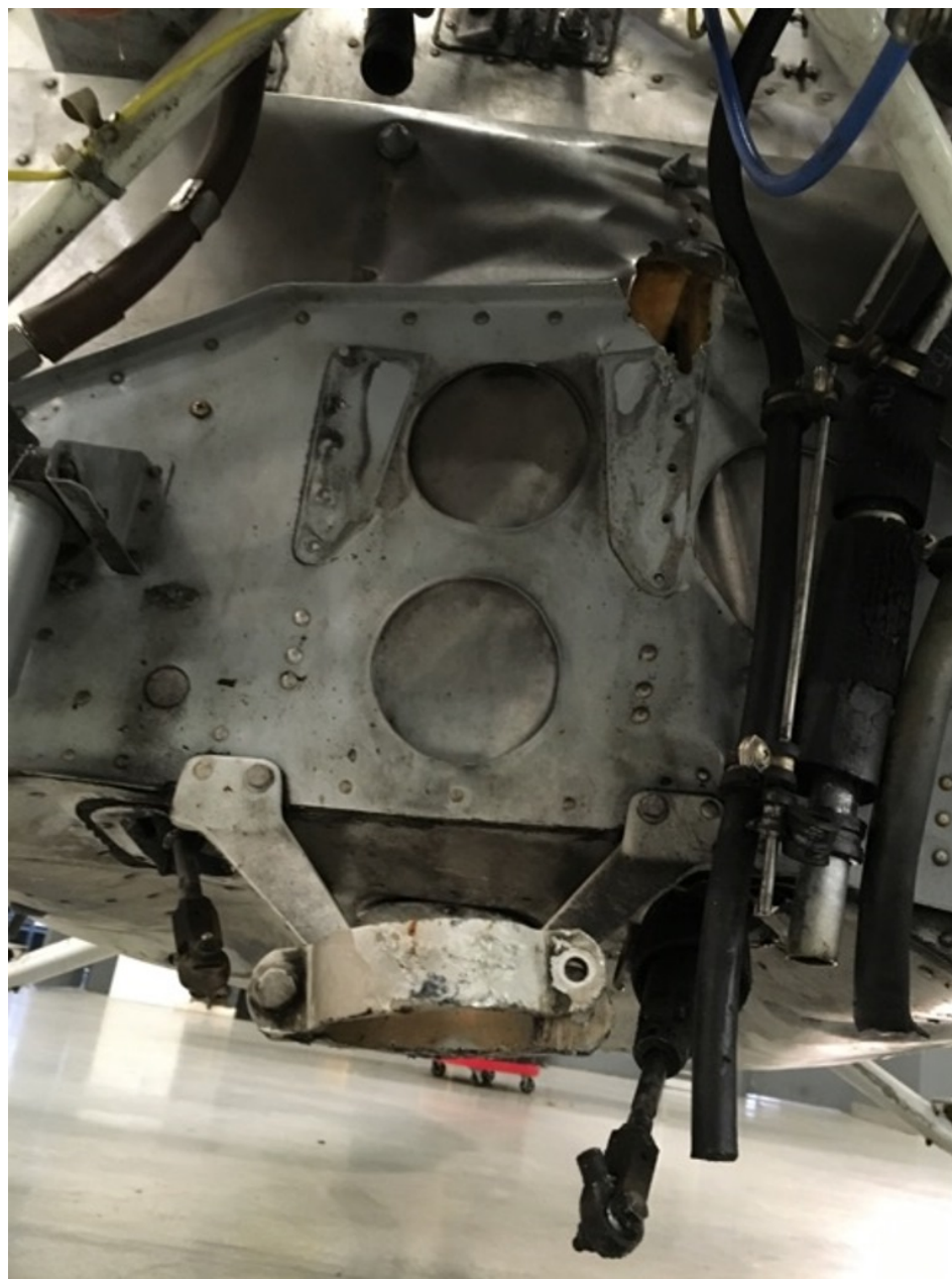
Photo 2 – View of damage to the firewall (Courtesy of FAA)
