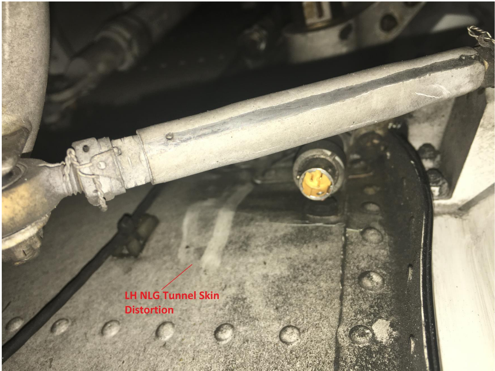
Photo 2 – View of nose landing gear tunnel (courtesy of the manufacturer)
