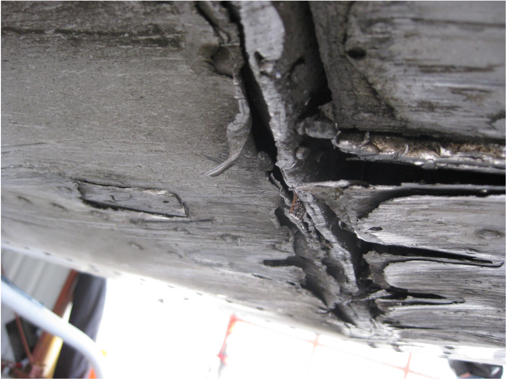
Photo 2 – Substantial Damage to the Underside of the Fuselage (Courtesy of FAA)
