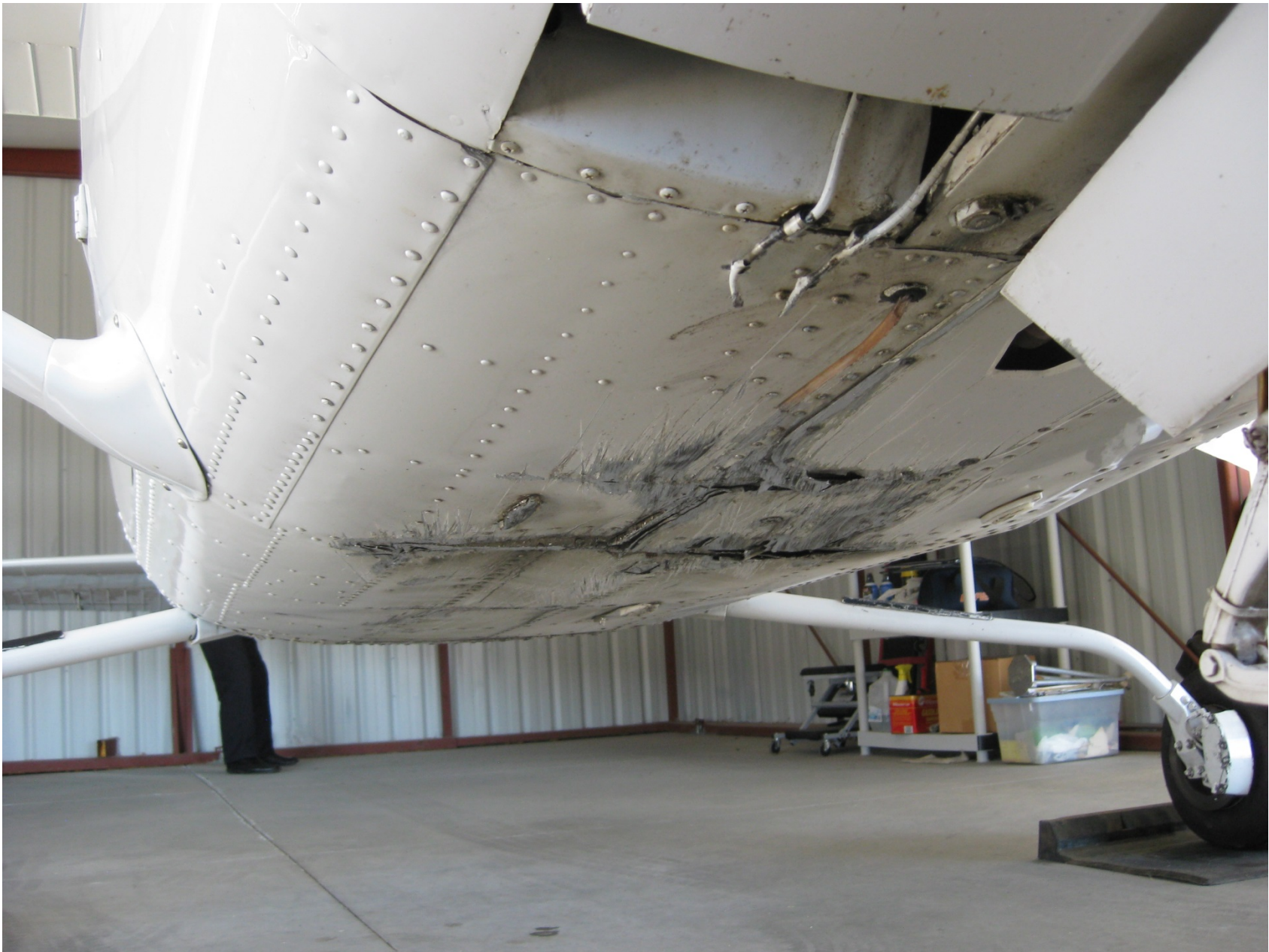
Photo 1 – Substantial Damage to the Fuselage (Courtesy of FAA)
