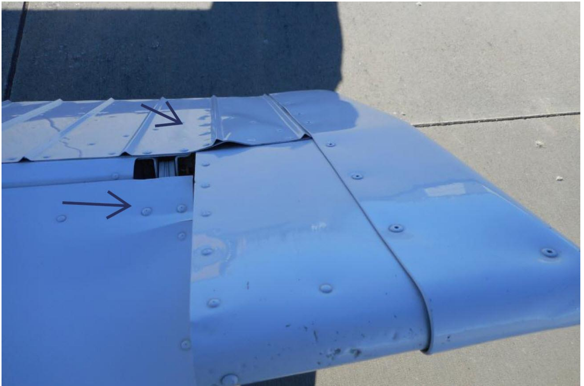
Photo 3 – Damage to left elevator and horizontal stabilizer (Courtesy of FAA)
