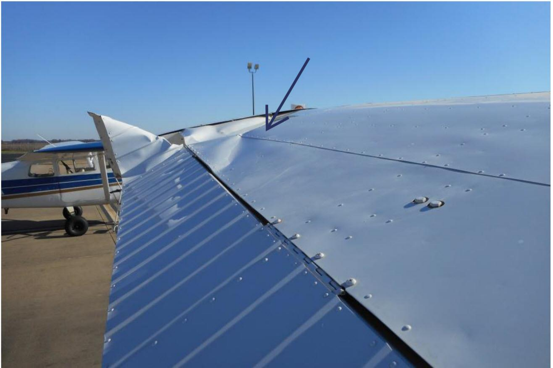
Photo 2 – Damage to left aileron and wing (Courtesy of FAA)
