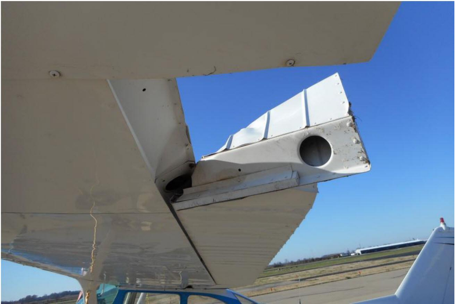
Photo 1 – Damage to left aileron (Courtesy of FAA)
