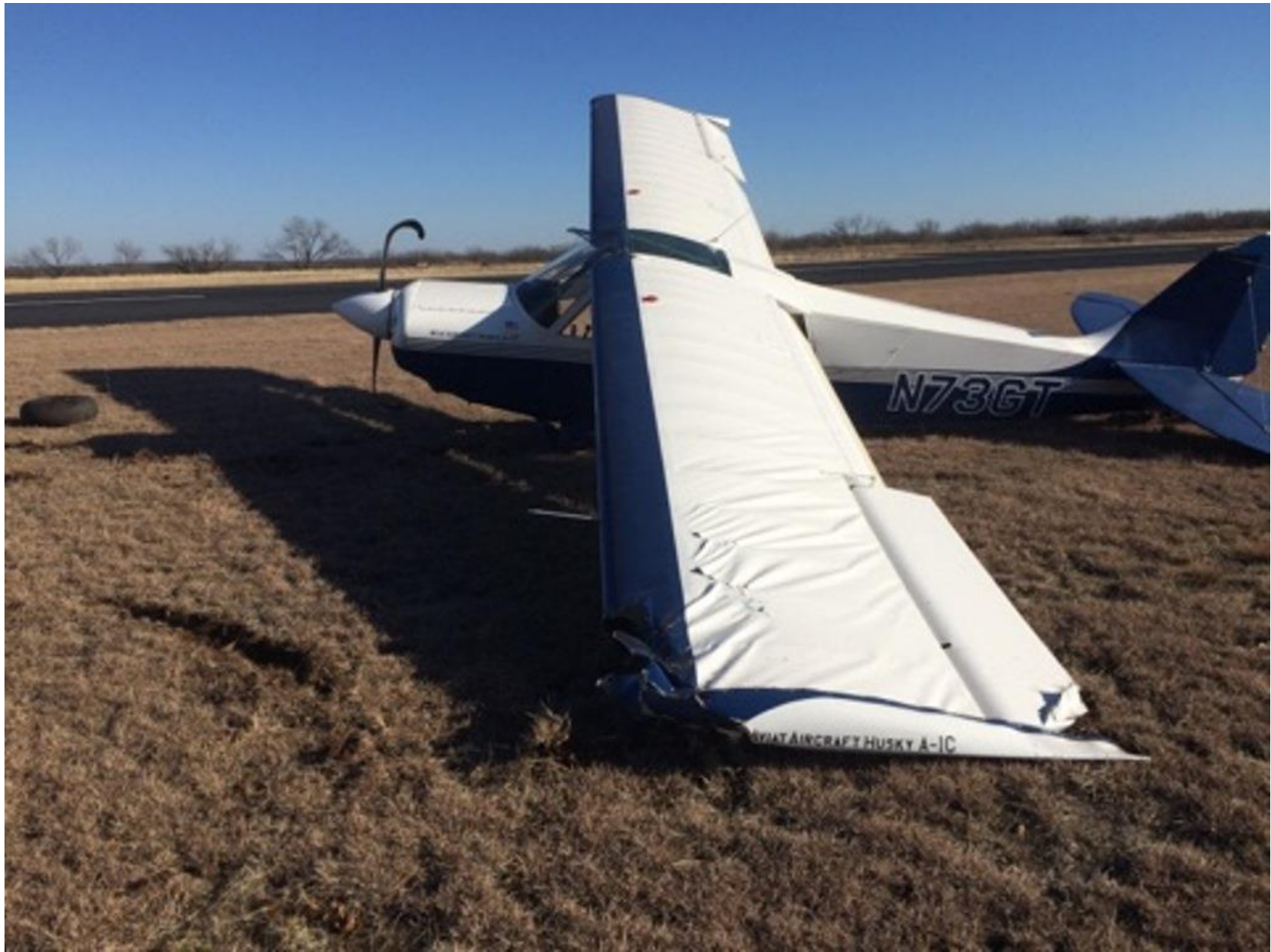
Photo 1 – Damage to left wing and aileron (Courtesy of pilot)
