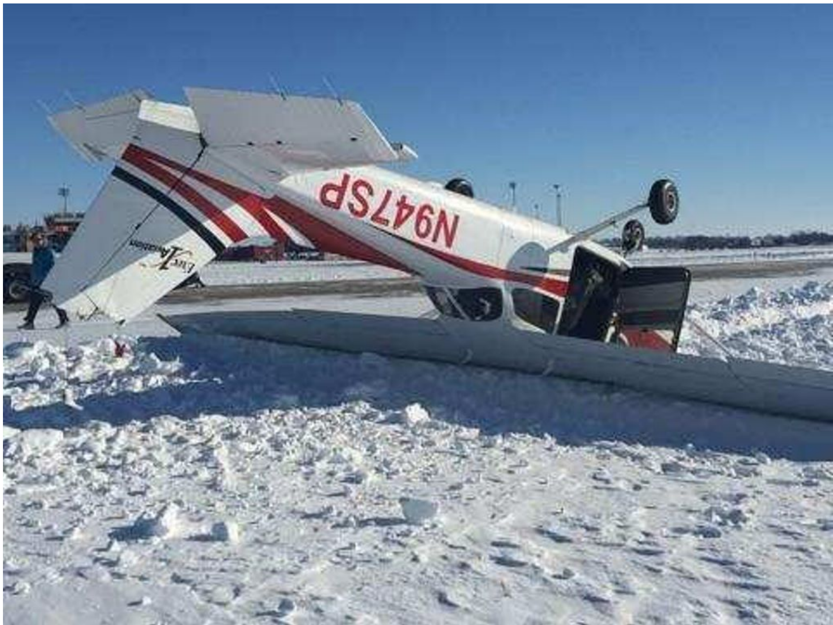
Photo 1 – View of damage to vertical stabilizer and rudder (Courtesy of FAA)
