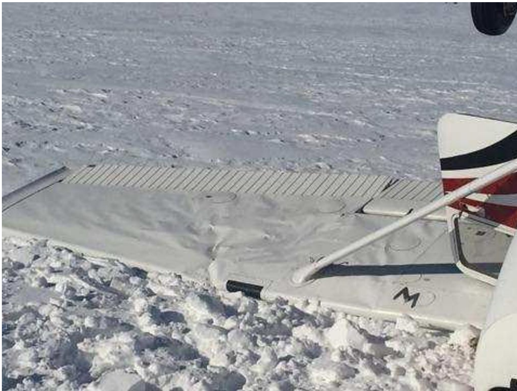
Photo 2 – View of damage to left wing spar (Courtesy of FAA)
