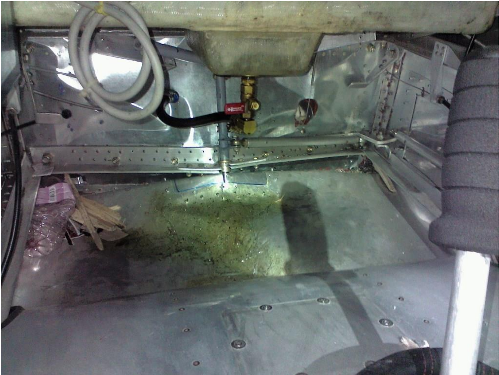
Photo 1 – Firewall damage from inside the cockpit (Courtesy of FAA)
