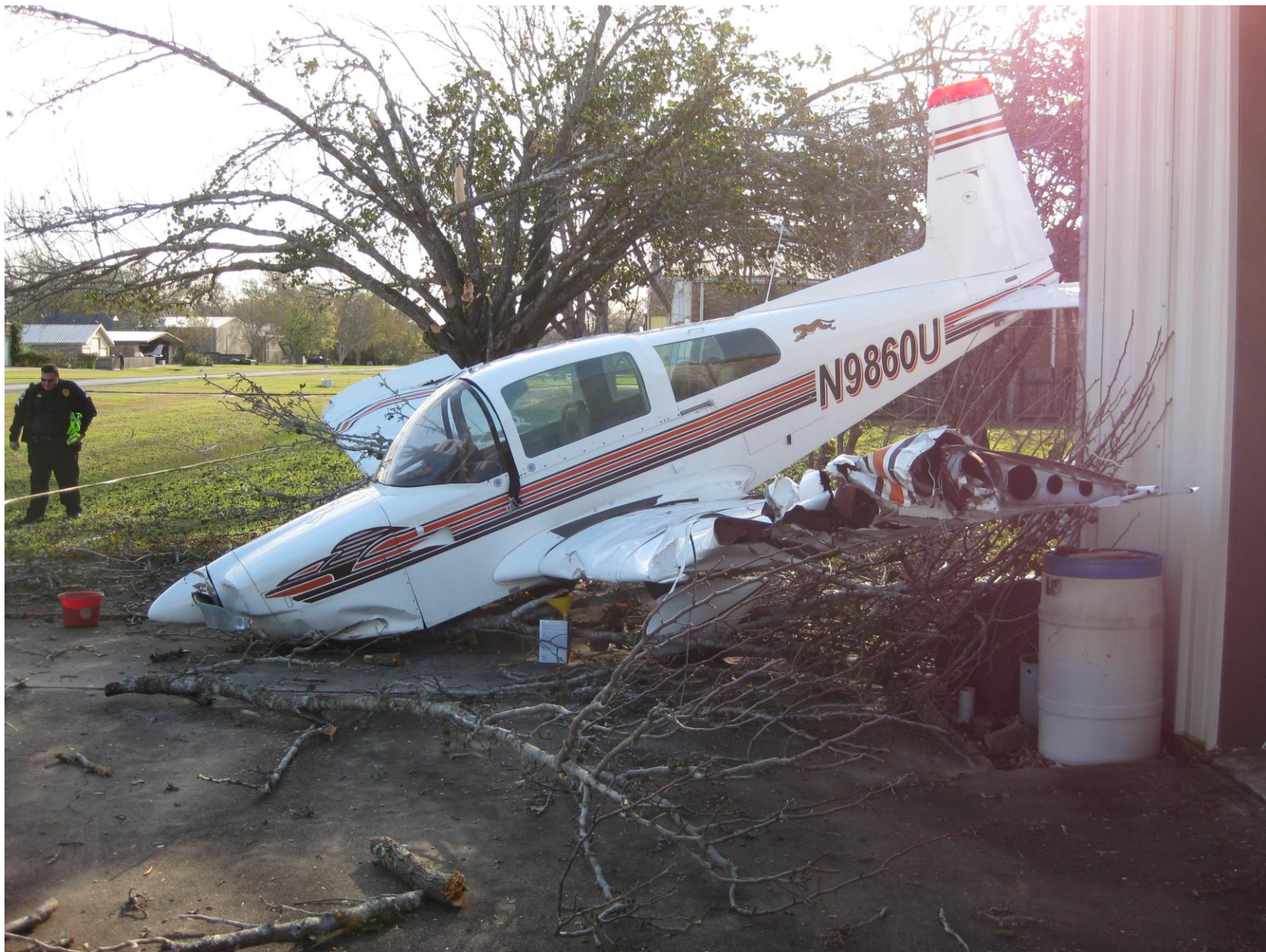
Photo 2 – Airplane with substantial damage to the left wing (Courtesy of FAA)
