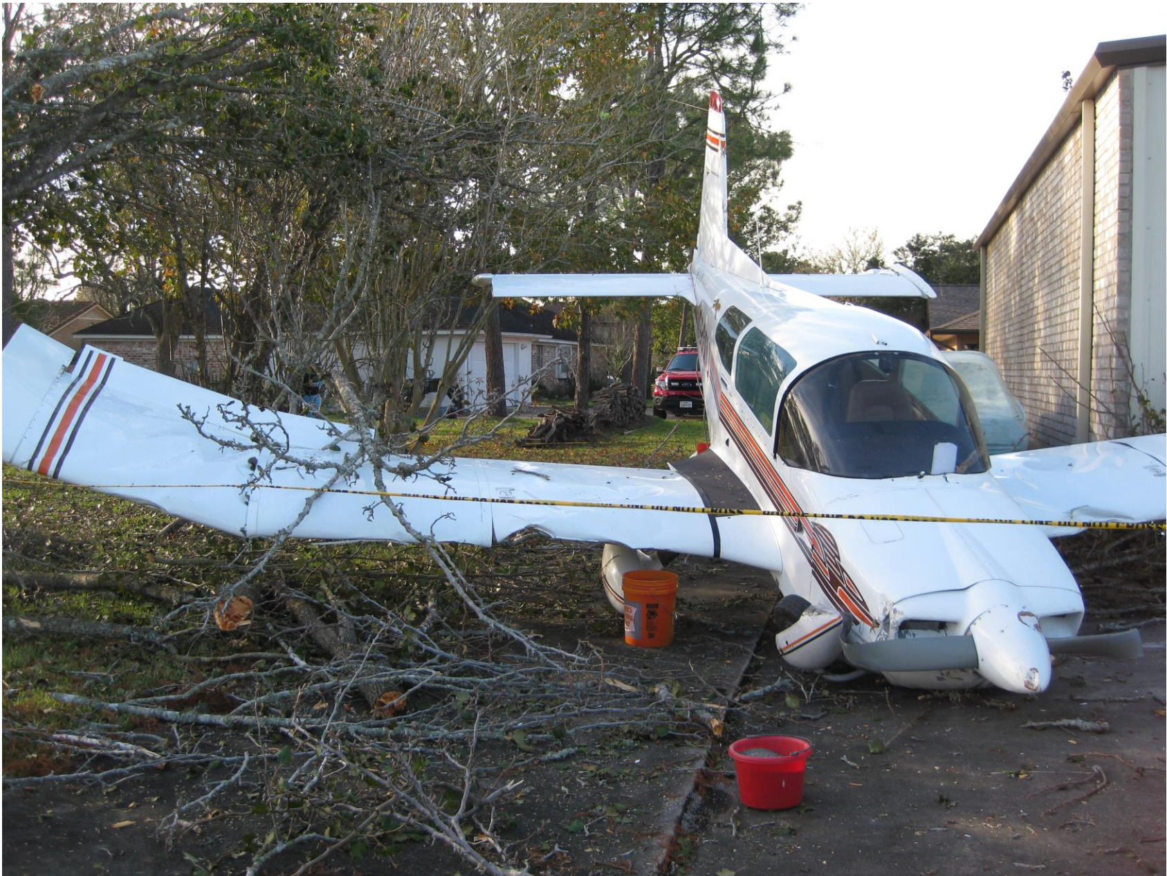
Photo 1 – Airplane with substantial damage to the right wing (Courtesy of FAA)
