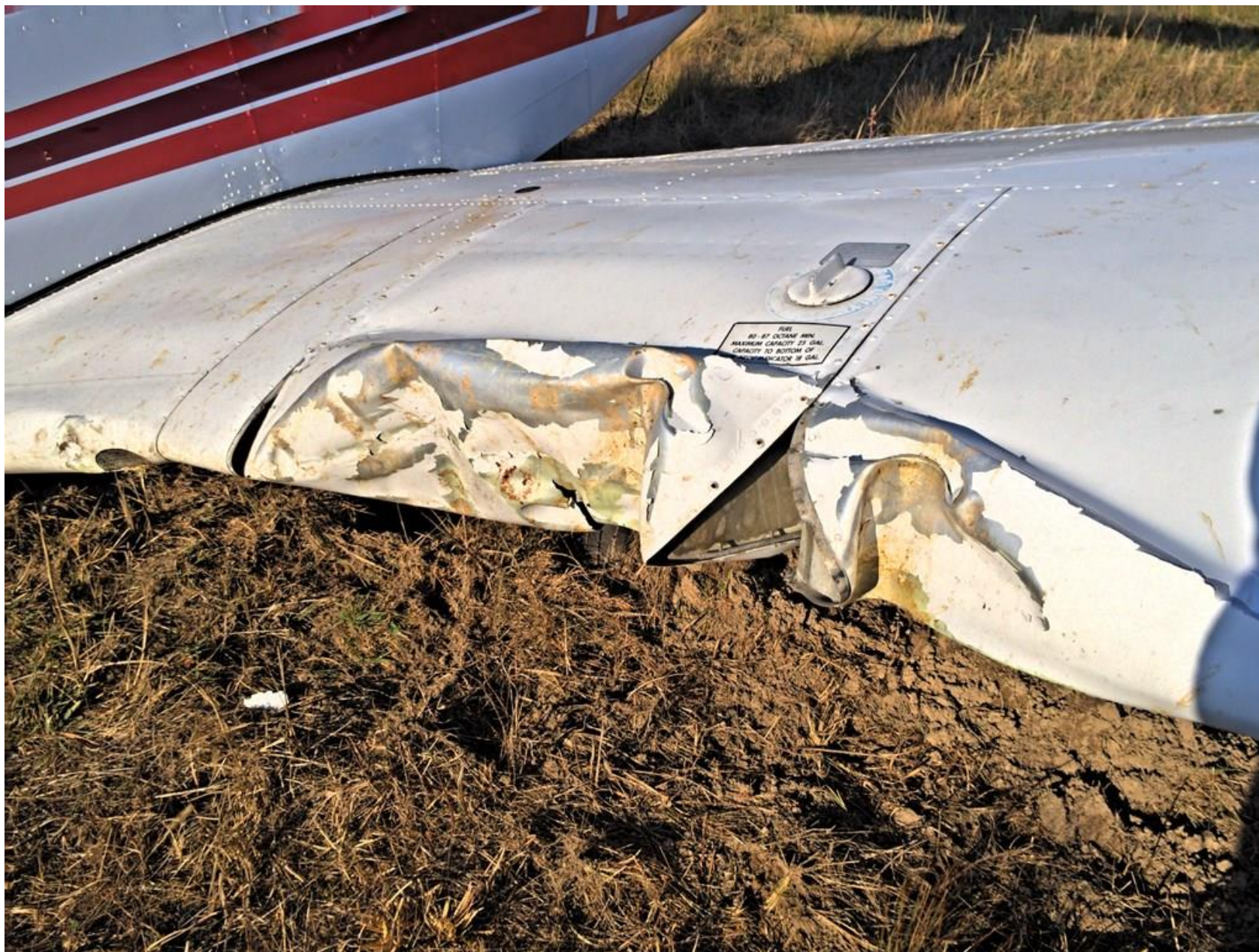
Photo 1 – Left wing leading edge impact damage after colliding with trees (Courtesy of FAA)
