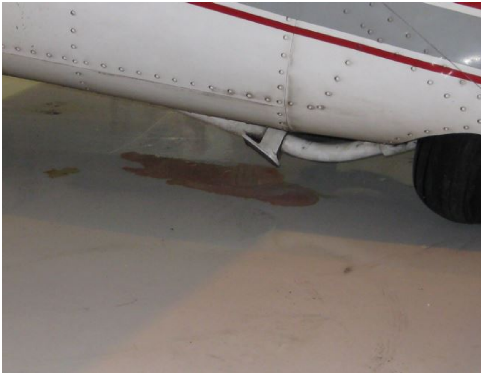
Photo 2 – Hydraulic Fluid Leak (Courtesy of FAA)
