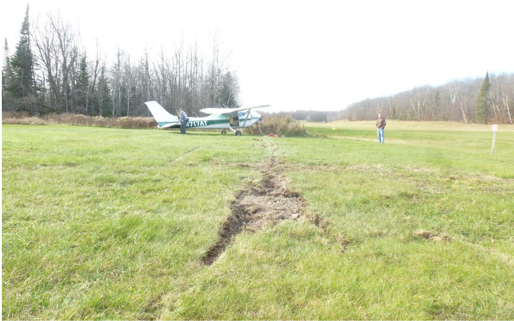
Photo 1 – View of initial impact point and ground scar leading up to main wreckage (photo courtesy of the FAA)
