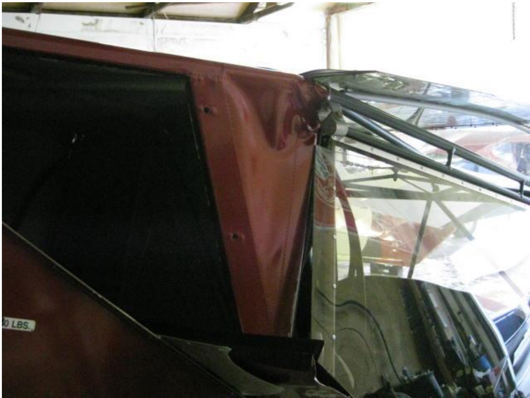
Photo 1 – Damage to truss structure at the right rear wing root attachment point (Courtesy of FAA)
