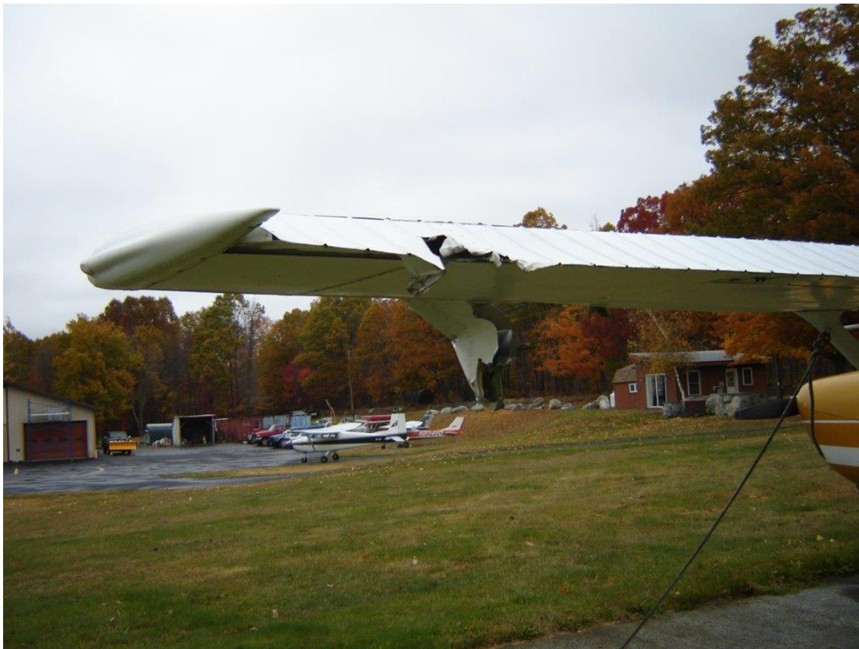
Photo 2 – Left Aileron (Courtesy of FAA)
