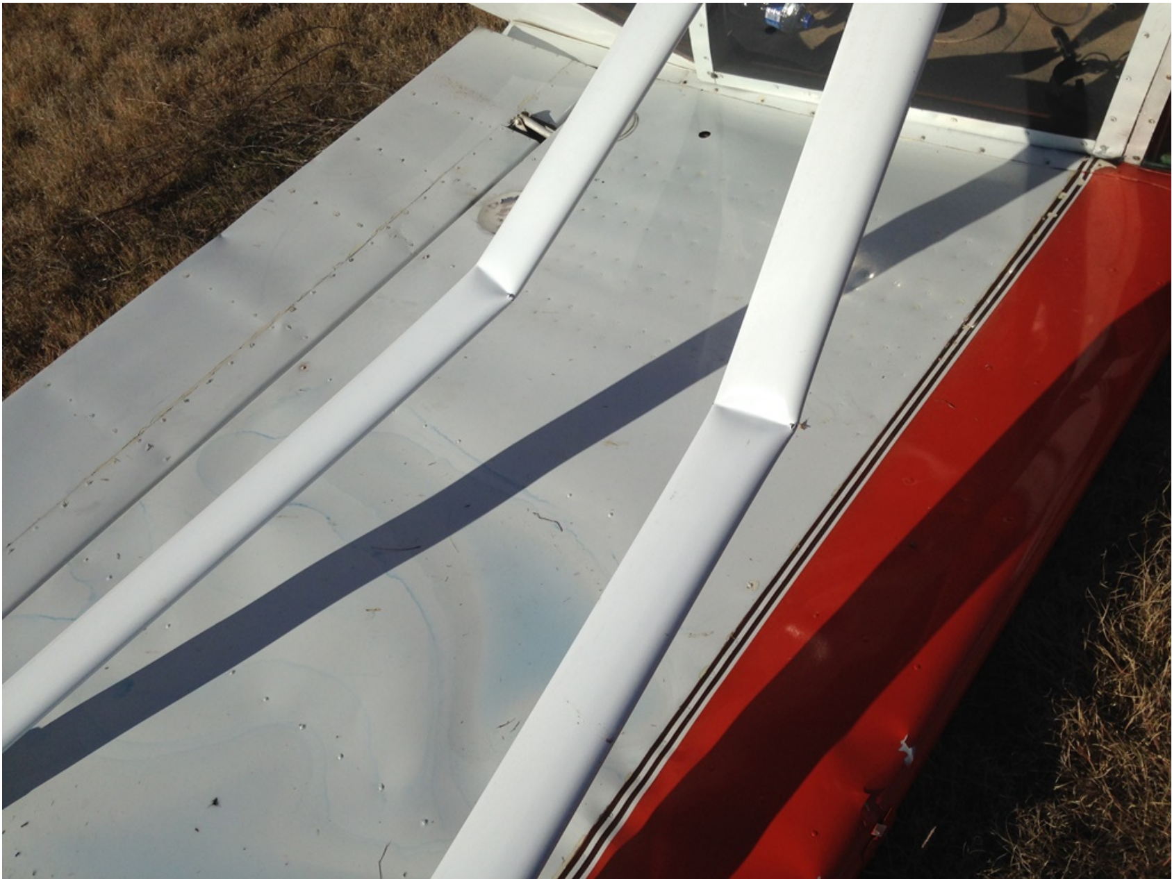
Photo 3 – View of damage to left wing struts (Courtesy of FAA)
