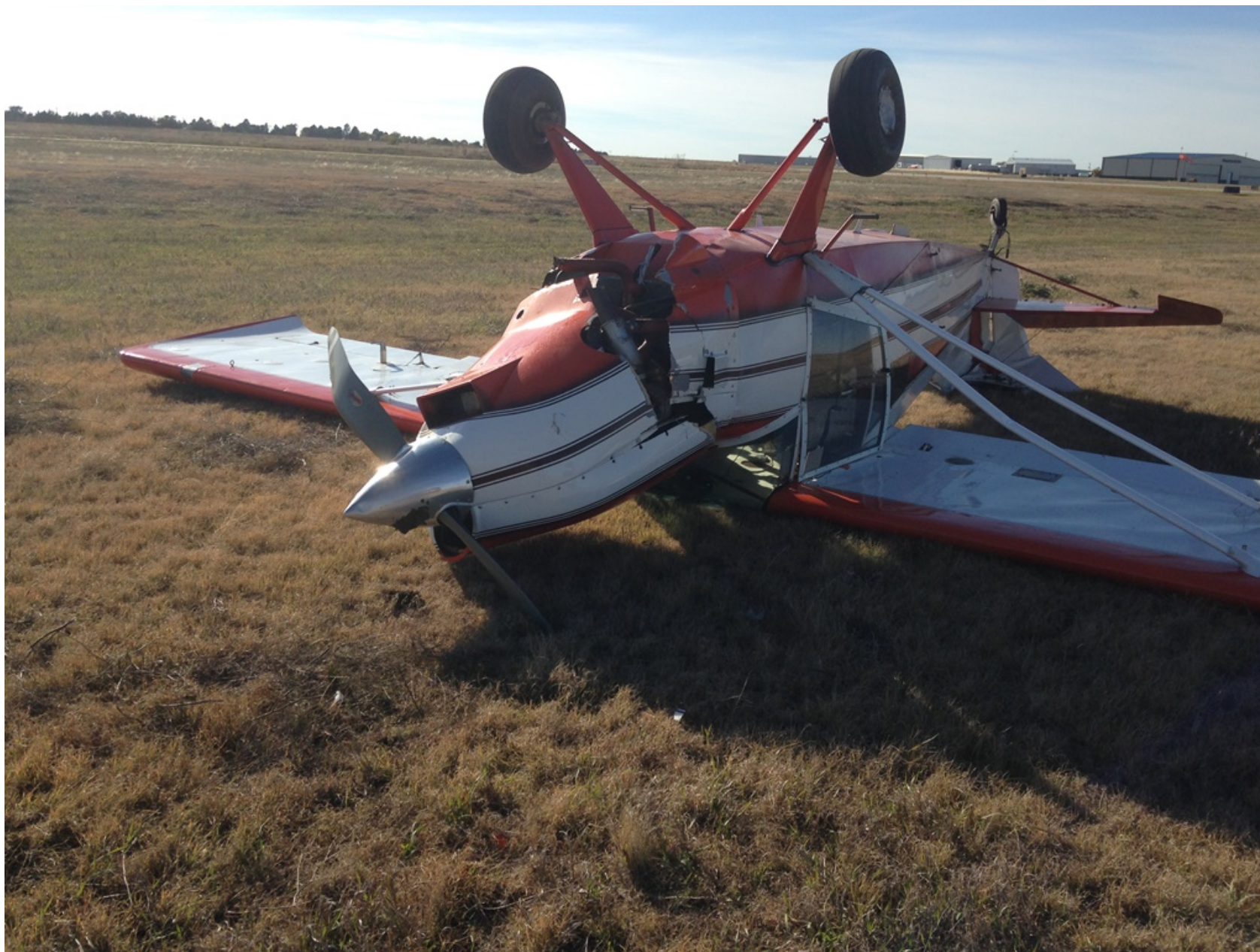
Photo 2 – View of damage to right wing strut (Courtesy of FAA)
