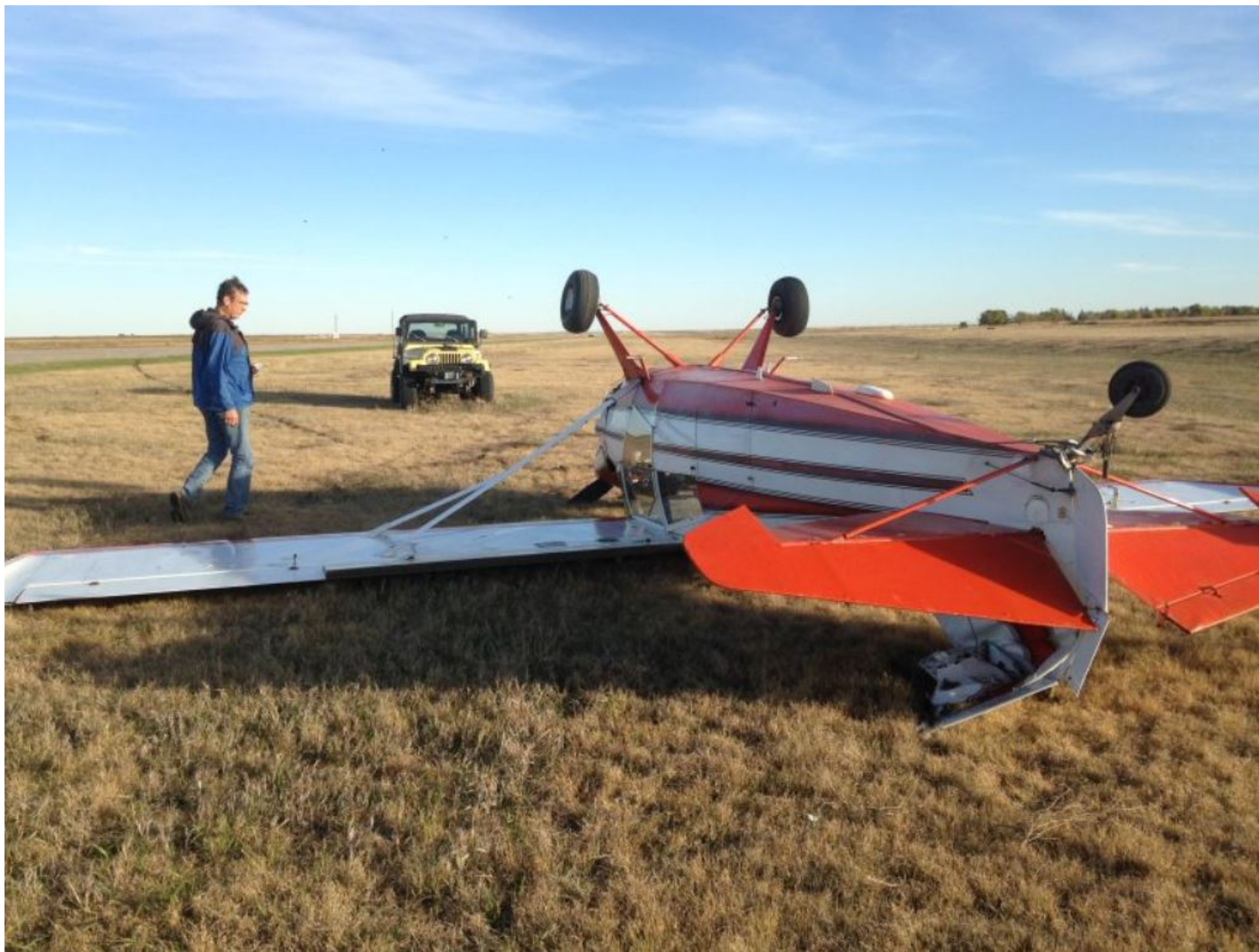
Photo 1 – View of damage to rudder and vertical stabilizer (Courtesy of FAA)
