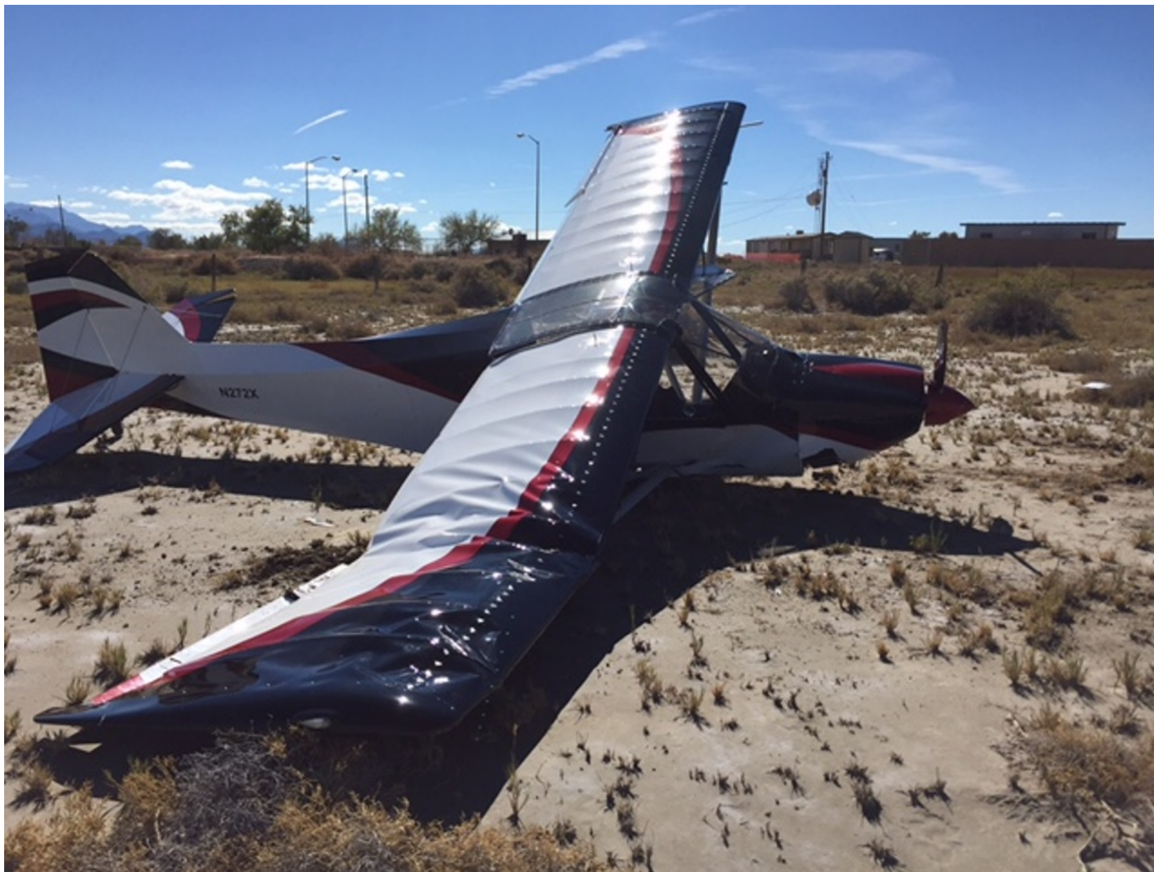
Photo 1 – View of substantial damage to right wing (Courtesy of FAA)
