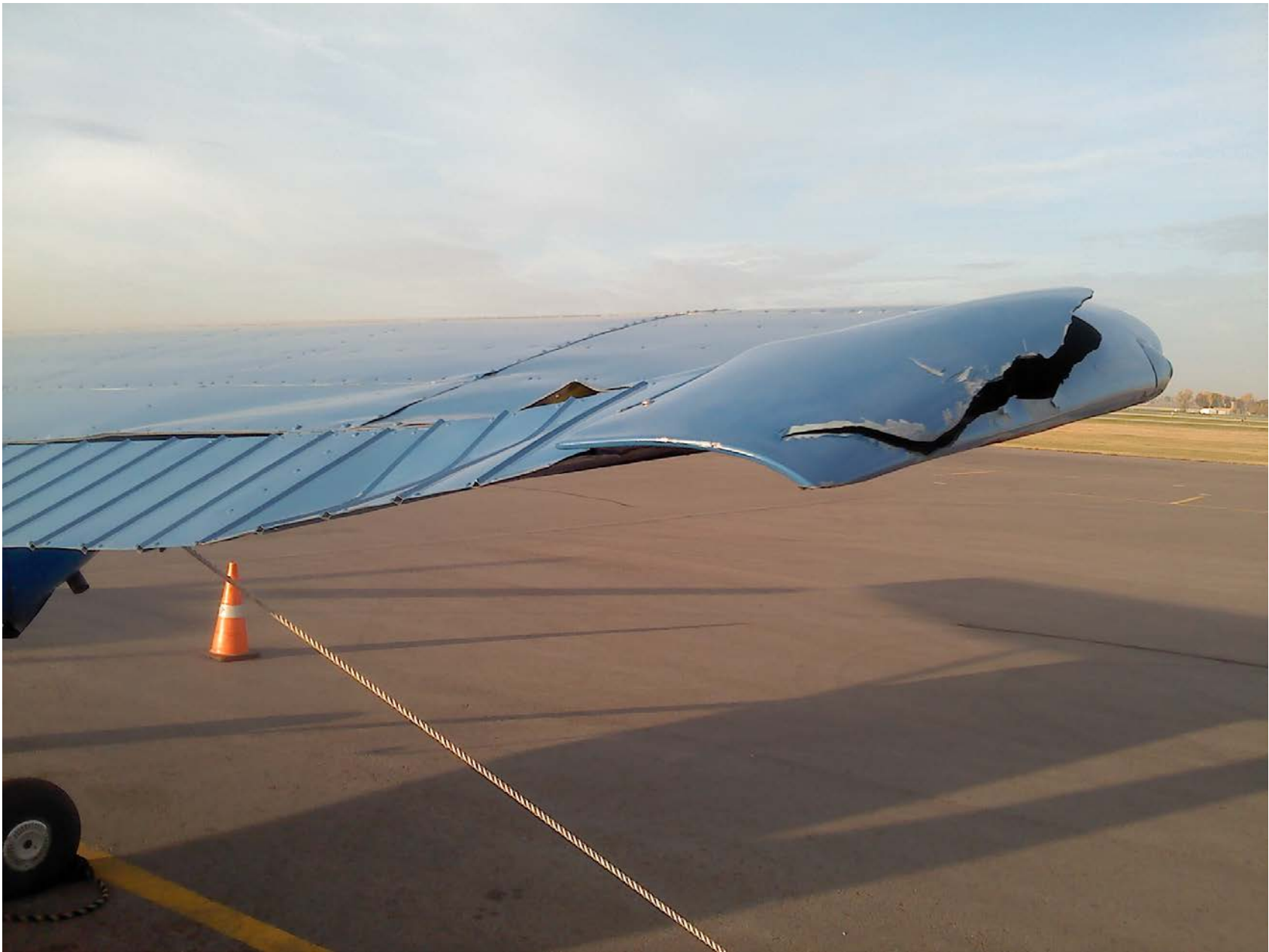
Photo 2 - View of right aileron damage (photo courtesy of the FAA)
