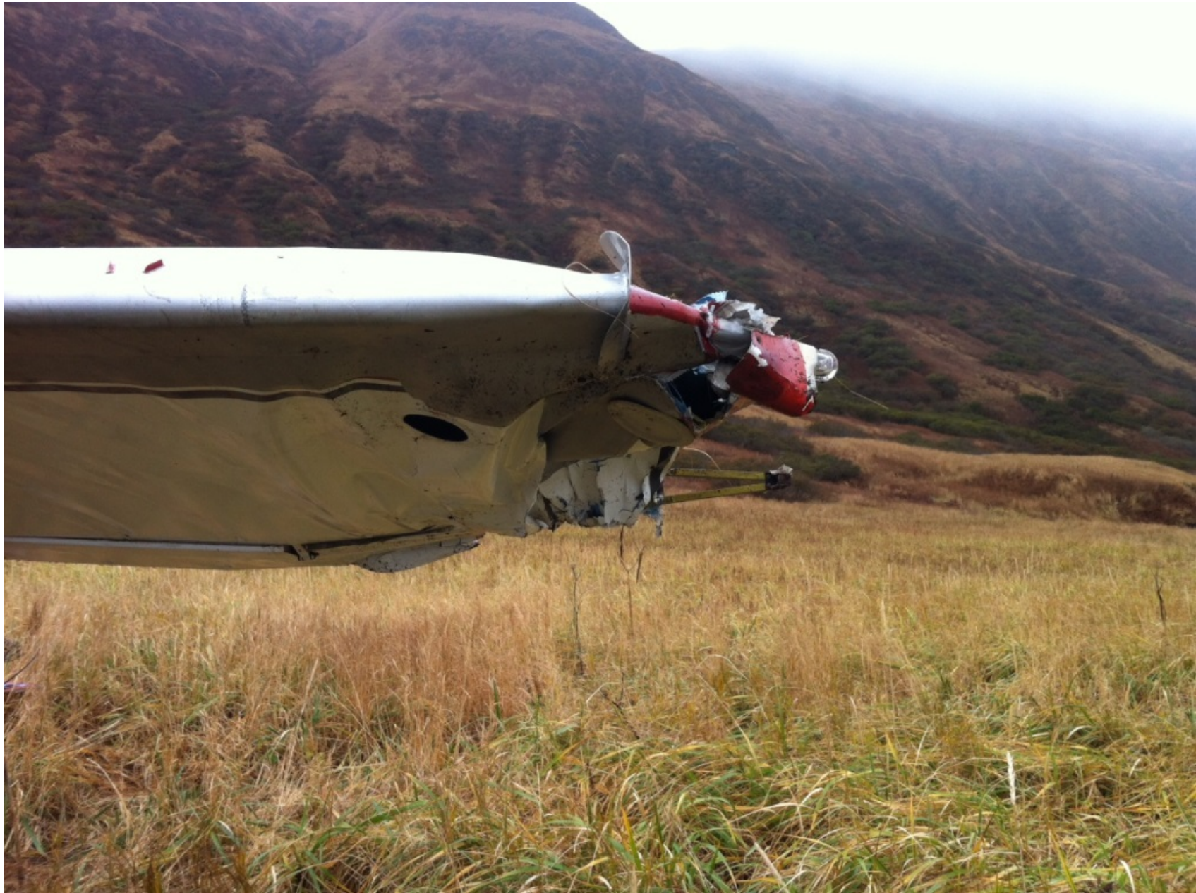
Photo 1 – View of substantial damage to left wing (Courtesy of Pilot)
