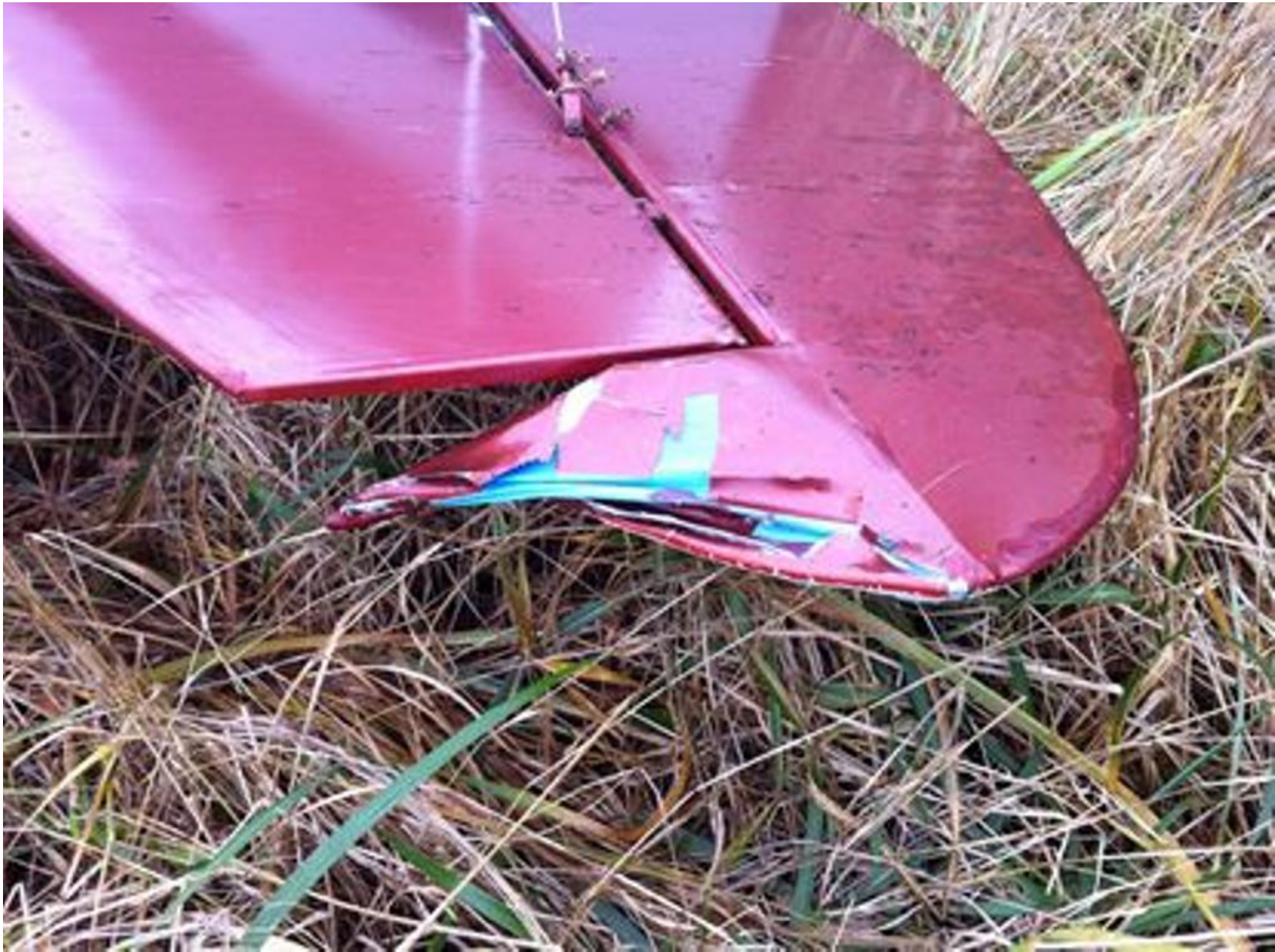
Photo 4 – View of damage to elevator (Courtesy of Pilot)
