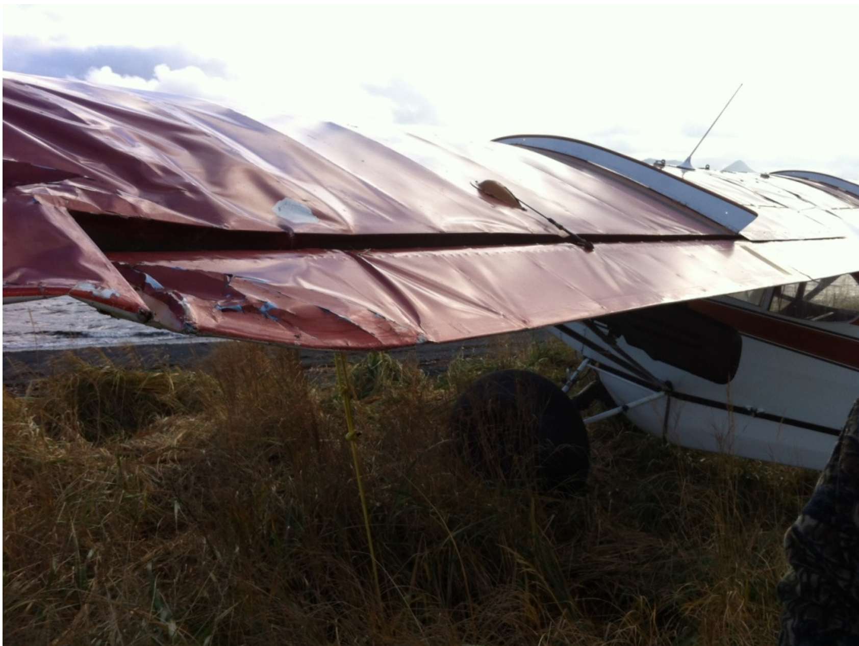
Photo 2 – View of substantial damage to aileron (Courtesy of Pilot)
