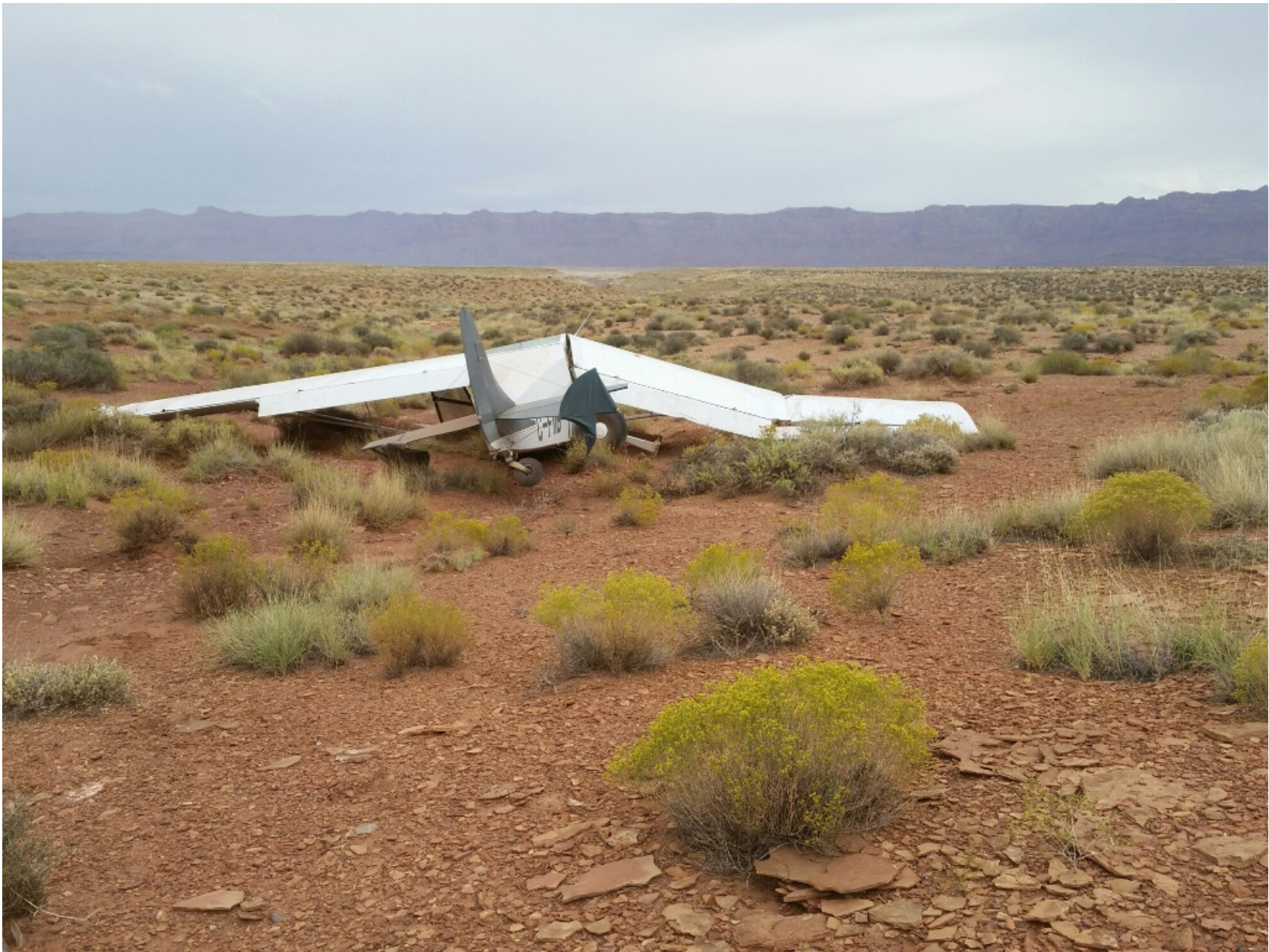
Photo 2 – View of substantial damage to empennage and right wing (Courtesy of FAA)
