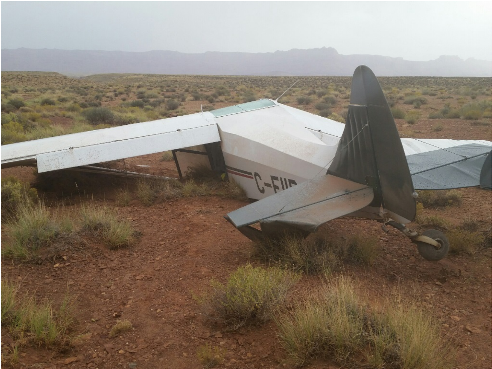
Photo 1 – View of substantial damage to empennage and left wing (Courtesy of FAA)
