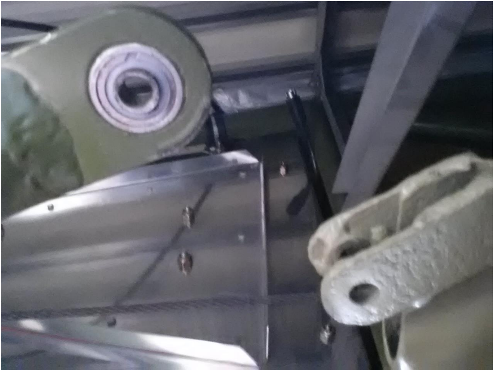
Photo 3 – Push-pull tube and cable attachment (Courtesy of FAA)
