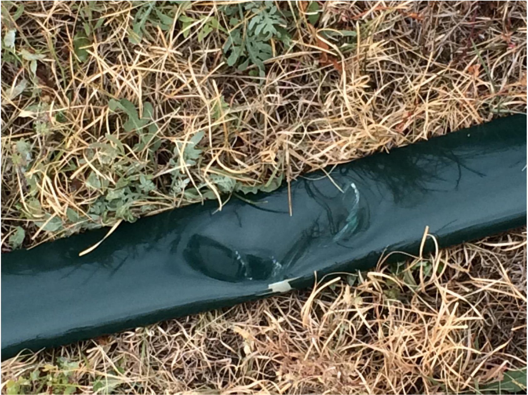
Photo 2 – Close up of damage to wing strut (Courtesy of NTSB)
