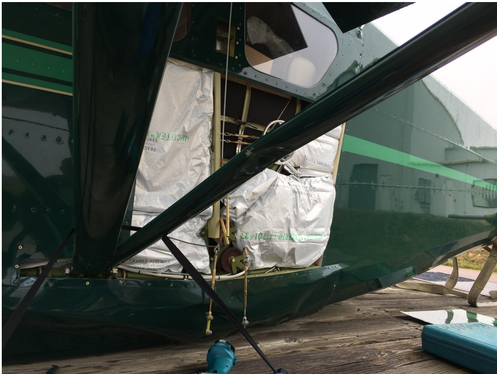
Photo 1 – Damage to left wing strut (Courtesy of NTSB)
