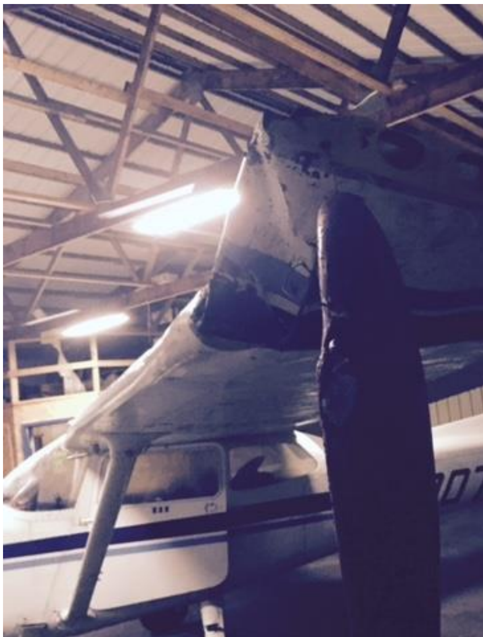
Photo 1 – Left wing damage (Courtesy of FAA)
