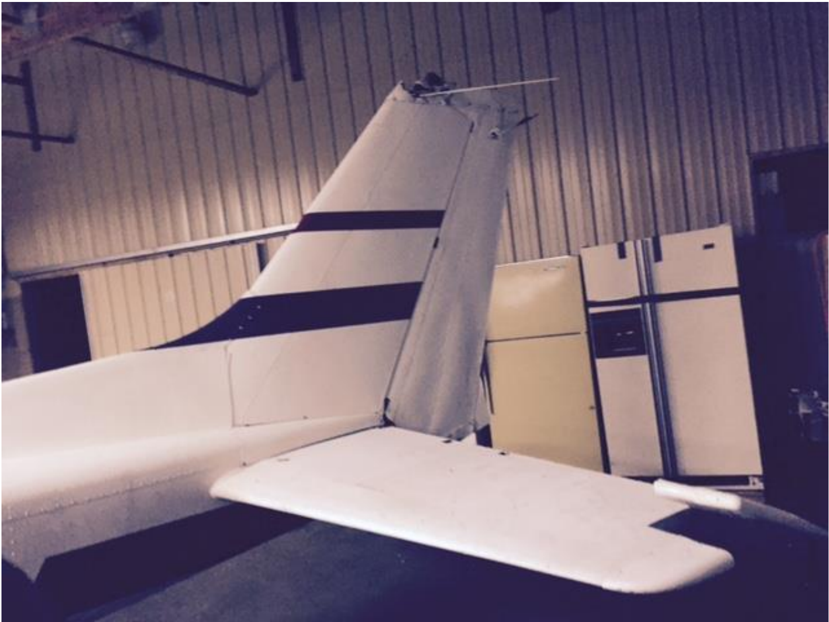
Photo 2 – Vertical Stabilizer and Rudder Damage (Courtesy of FAA)
