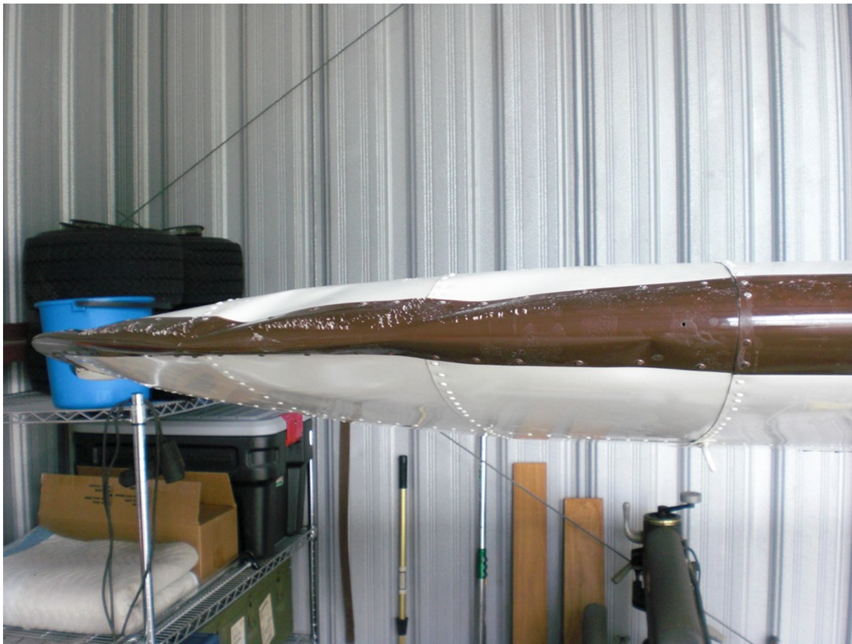
Photo 3 – View of damage to outboard right wing (Courtesy of FAA)
