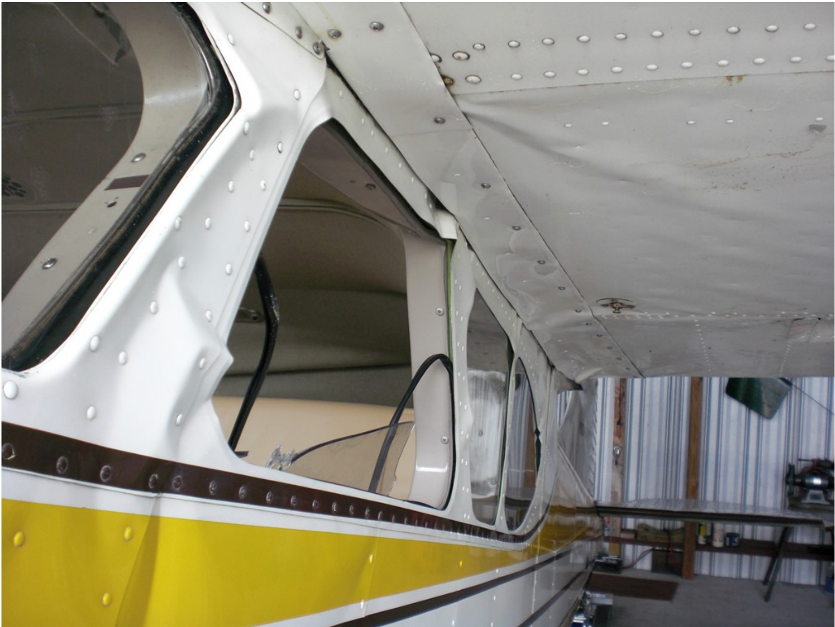
Photo 2 – View of substantial damage to fuselage and left inboard wing (Courtesy of FAA)
