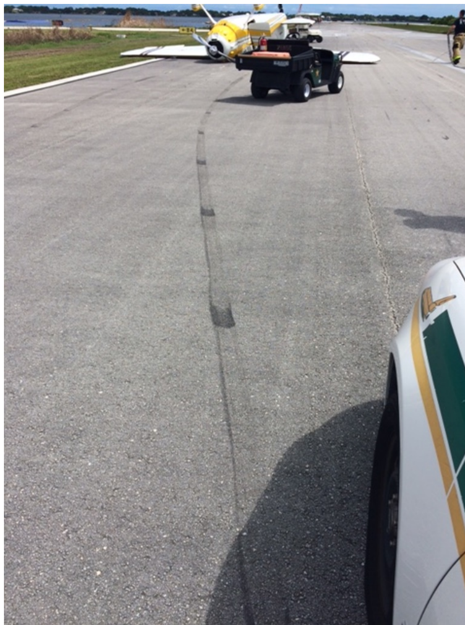
Photo 4 - View of right tire skid marks (Courtesy of FAA)
