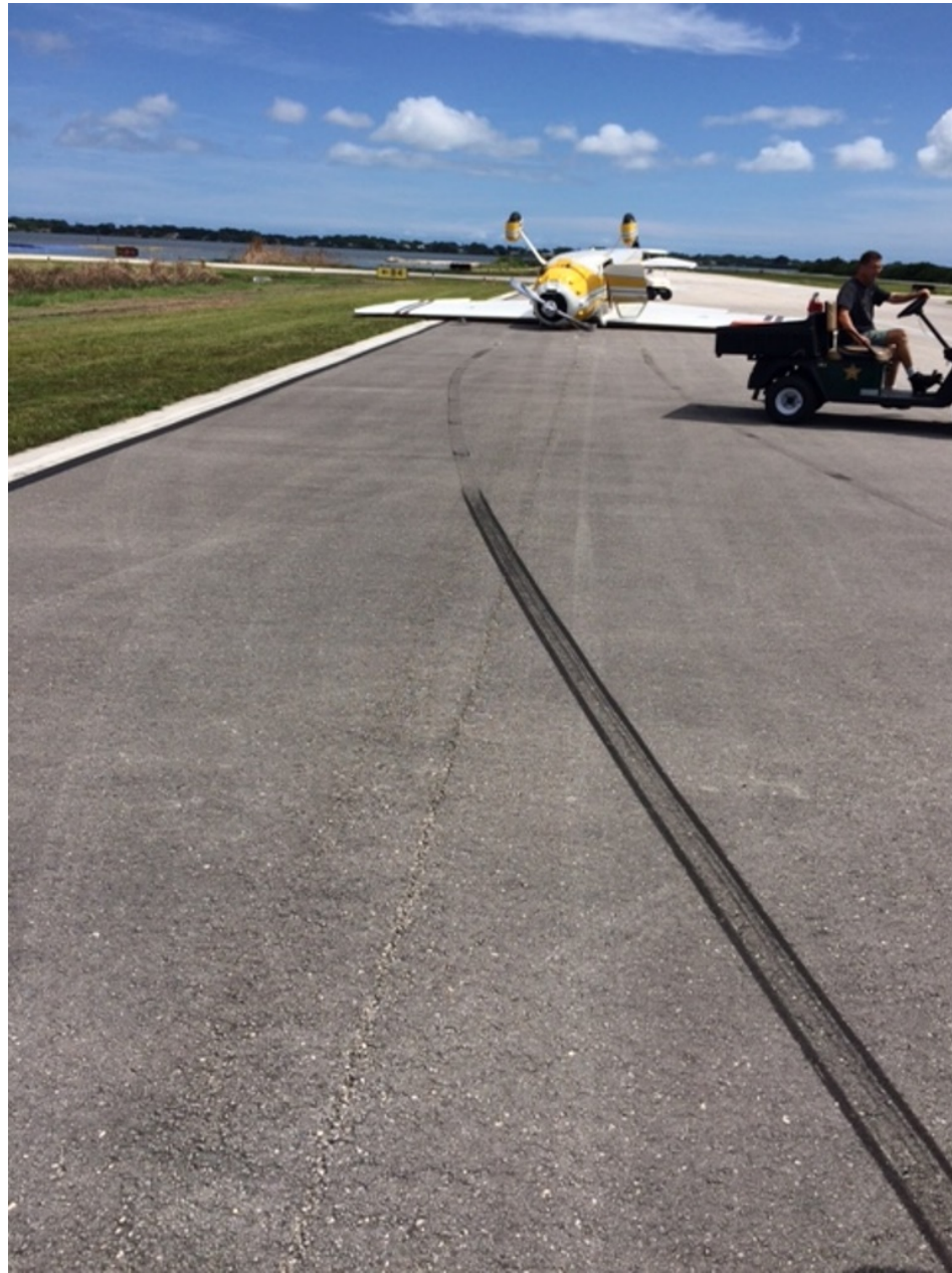
Photo 5 - View of left tire skid marks (Courtesy of FAA)
