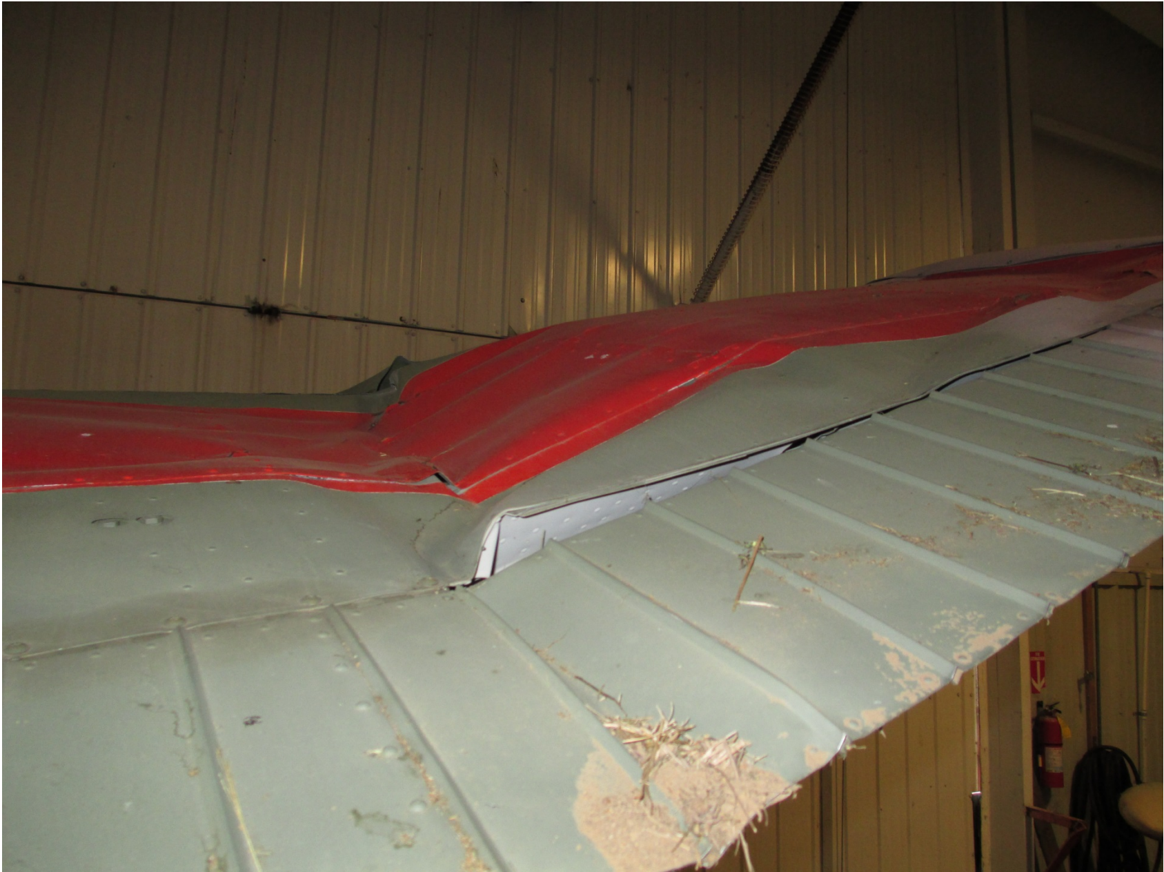
Photo 1 – Right Wing Damage (Courtesy of FAA)
