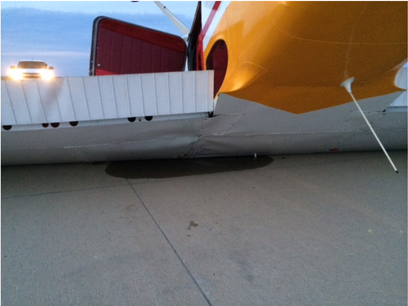
Photo 1 – View of right wing damage (courtesy of the FAA)
