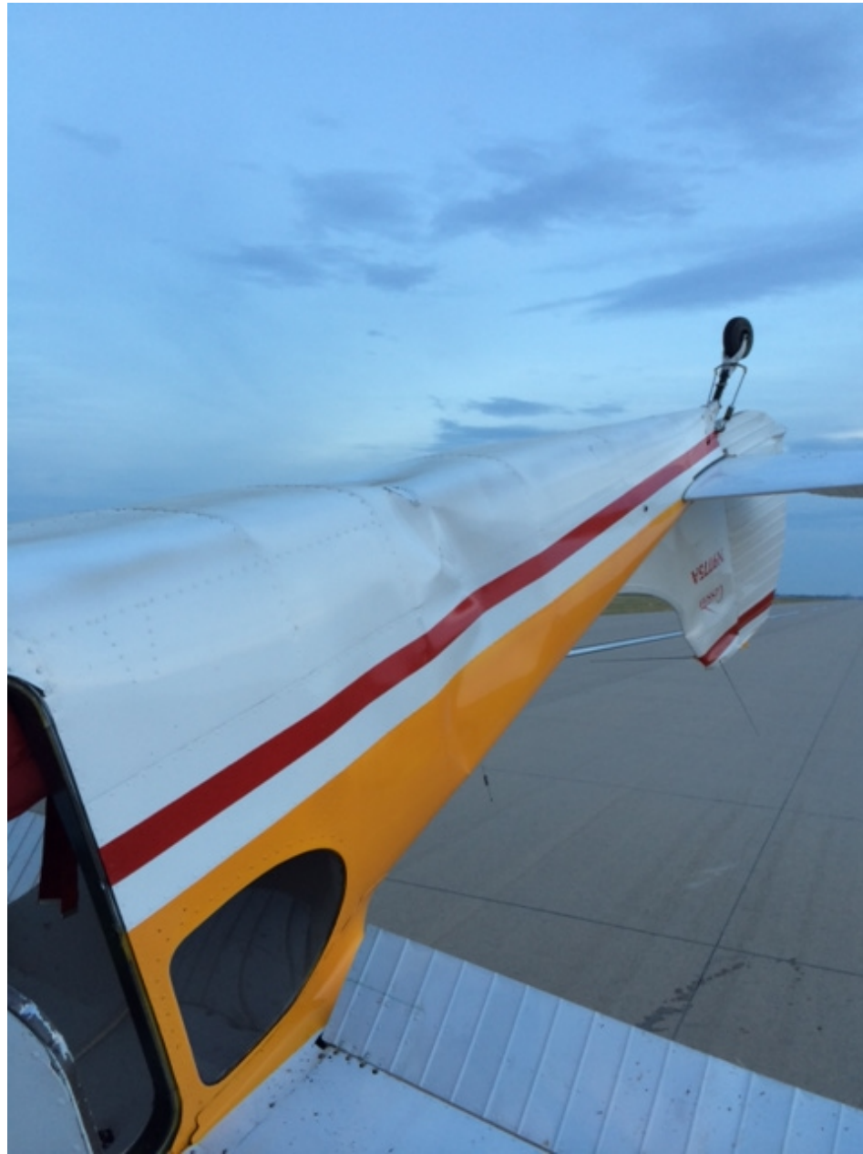
Photo 2 - View of fuselage damage (courtesy of the FAA)
