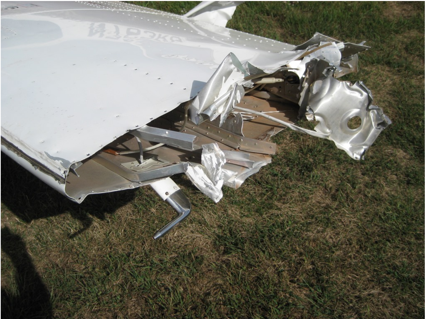
Photo 2 -View of substantial damage to left wing (Courtesy of FAA)
