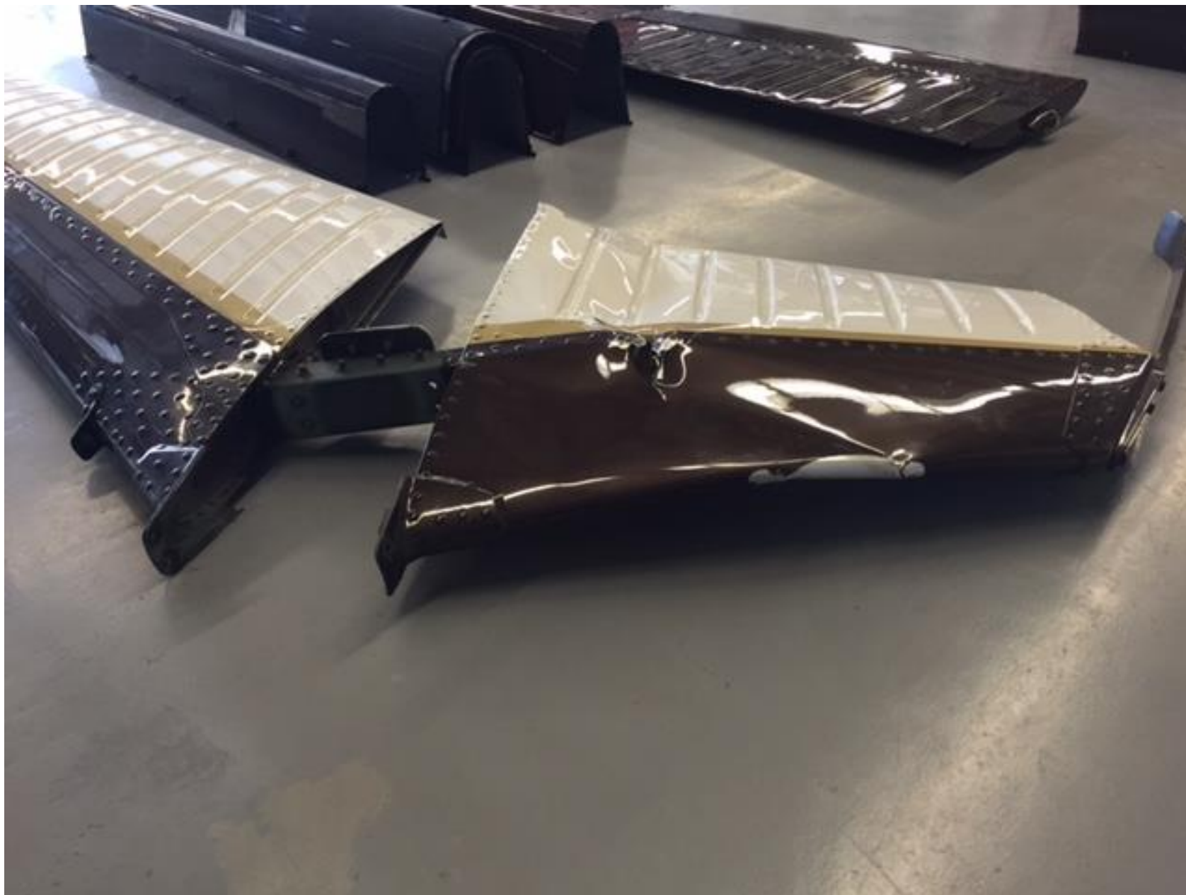
Photo 4 – View of vertical fin (photo courtesy of the Utah Highway Patrol Aero Bureau)
