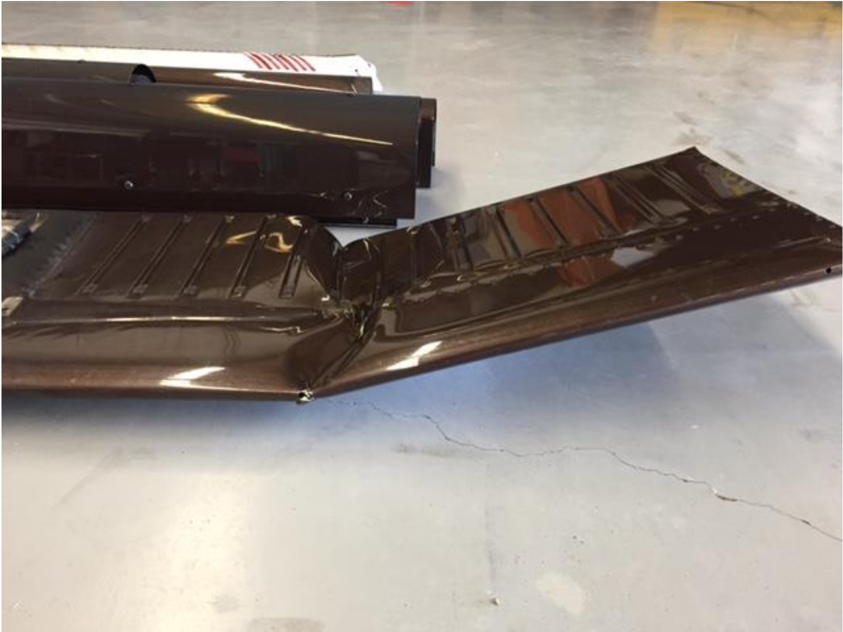
Photo 3 – View of horizontal stabilizer (photo courtesy of the Utah Highway Patrol Aero Bureau)
