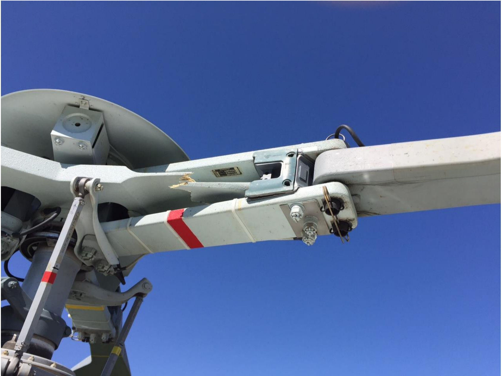
Photo 1 – View of Starflex assembly (photo courtesy of the Utah Highway Patrol Aero Bureau)
