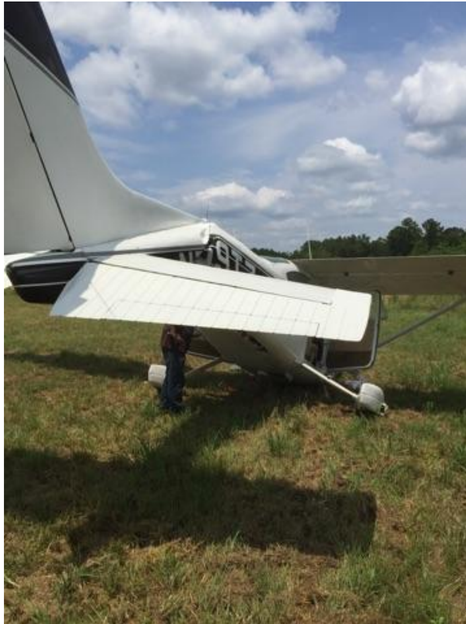
Photo 2 - View of fuselage damage from the rear (photo courtesy of the FAA)
